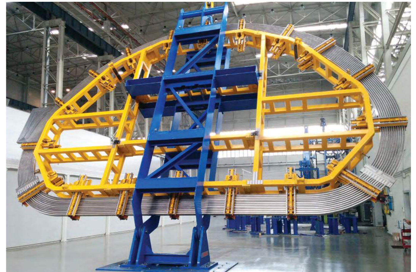
Overview of the SIMIC facility in Italy, Porto Marghera, while works of radial plate tilting are being carried out
