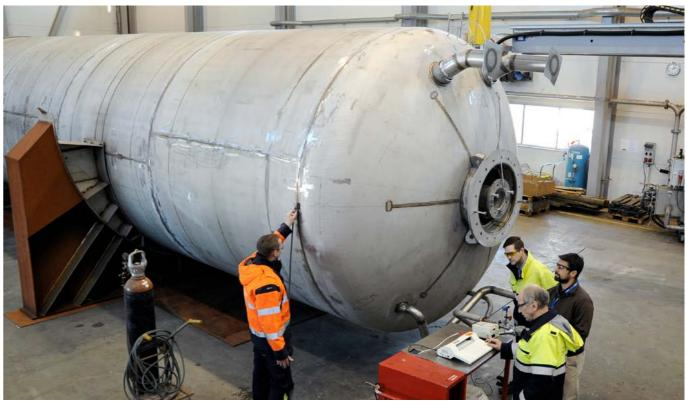
CryoAB technicians carrying out the liquid helium leak test on the inner-tank. It took almost half a day to inspect roughly 500 m of linear welds. February 2016
