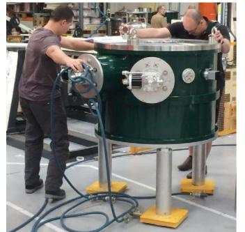
The magnet which will be joined to the gyrotron prototype and tested at Swiss Plasma Center
