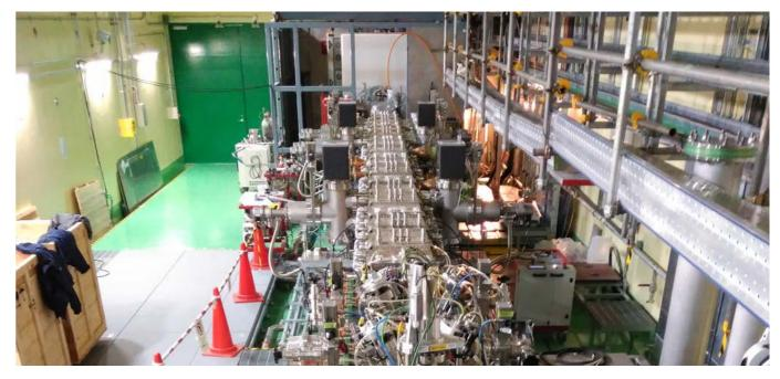
Installing the Radio Frequency Quadrupole and Injector already in position in IFMIF/EVEDA, Rokkasho, Japan
