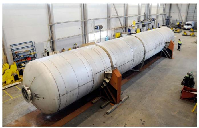
The liquid helium inner-tank, designed and manufactured by CryoAB, part of the contract signed between Air Liquide Global and EC Solutions and F4E, February 2016
