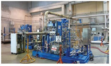
Turbo booster turbine able to generate 500 KW of cooling power fully assembled for testing at Cryostar
