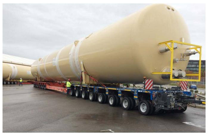
One of the two quench tanks stored at the ITER worksite. Manufactured by Air Liquide and their subcontractor Chart Ferox, it is 35 m long and has a diameter of 4.5 m. It weighs approximately 160 T.
