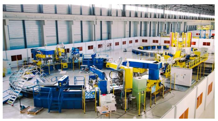
Winding tooling at the Poloidal Field coils Facility where cleaning, sandblasting, bending, insulation and wrapping of the conductor will be performed, Cadarache. August 2016
