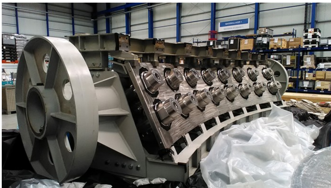
Figure 3: The triangular support subassembly for the fourth segment for the fifth Vacuum Vessel sector, manufactured by Mangiarotti in Italy and electron-beam welded at Pro-beam in Germany
