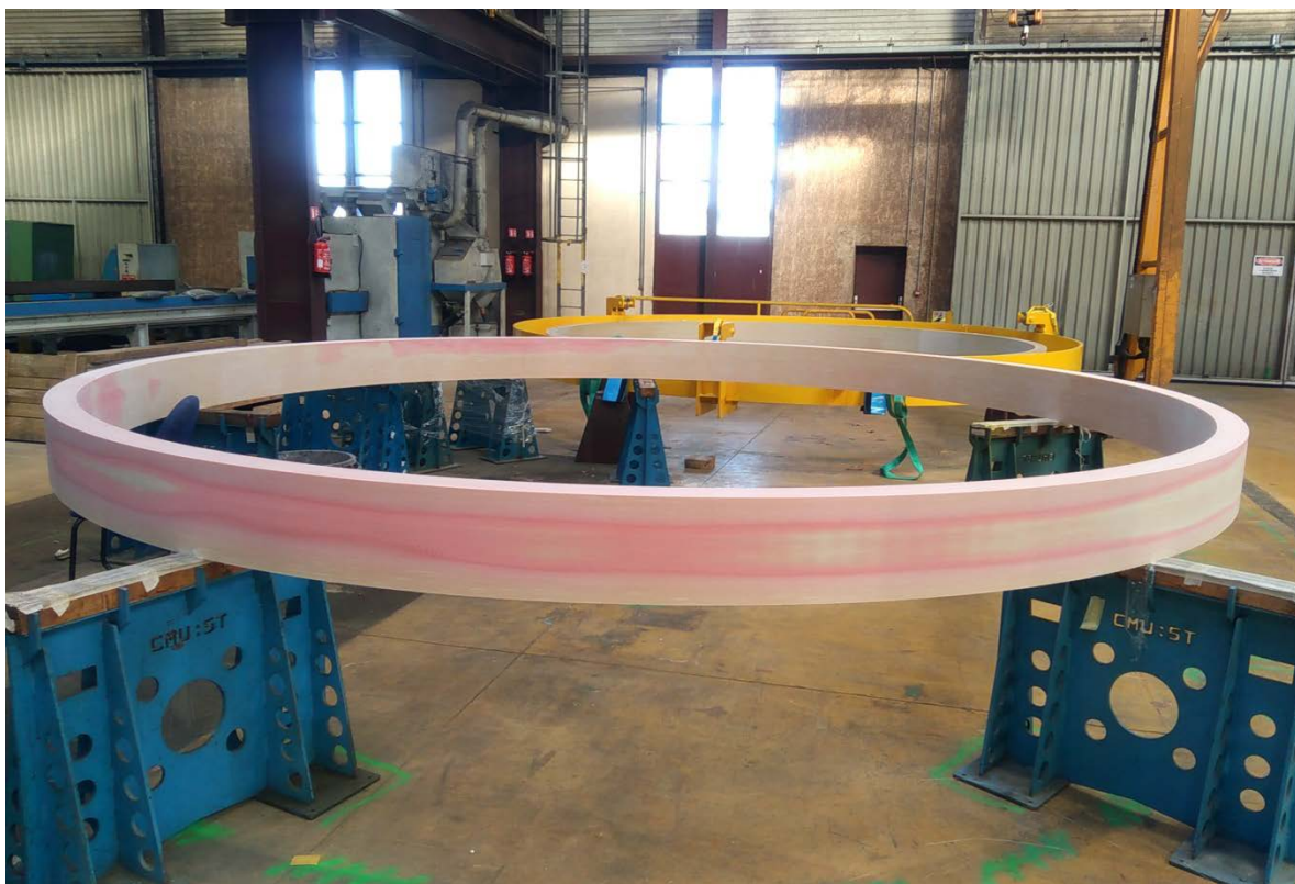
Figure 7: Pre-Compression Ring slice after machining, manufactured with pultrusion technology, France
