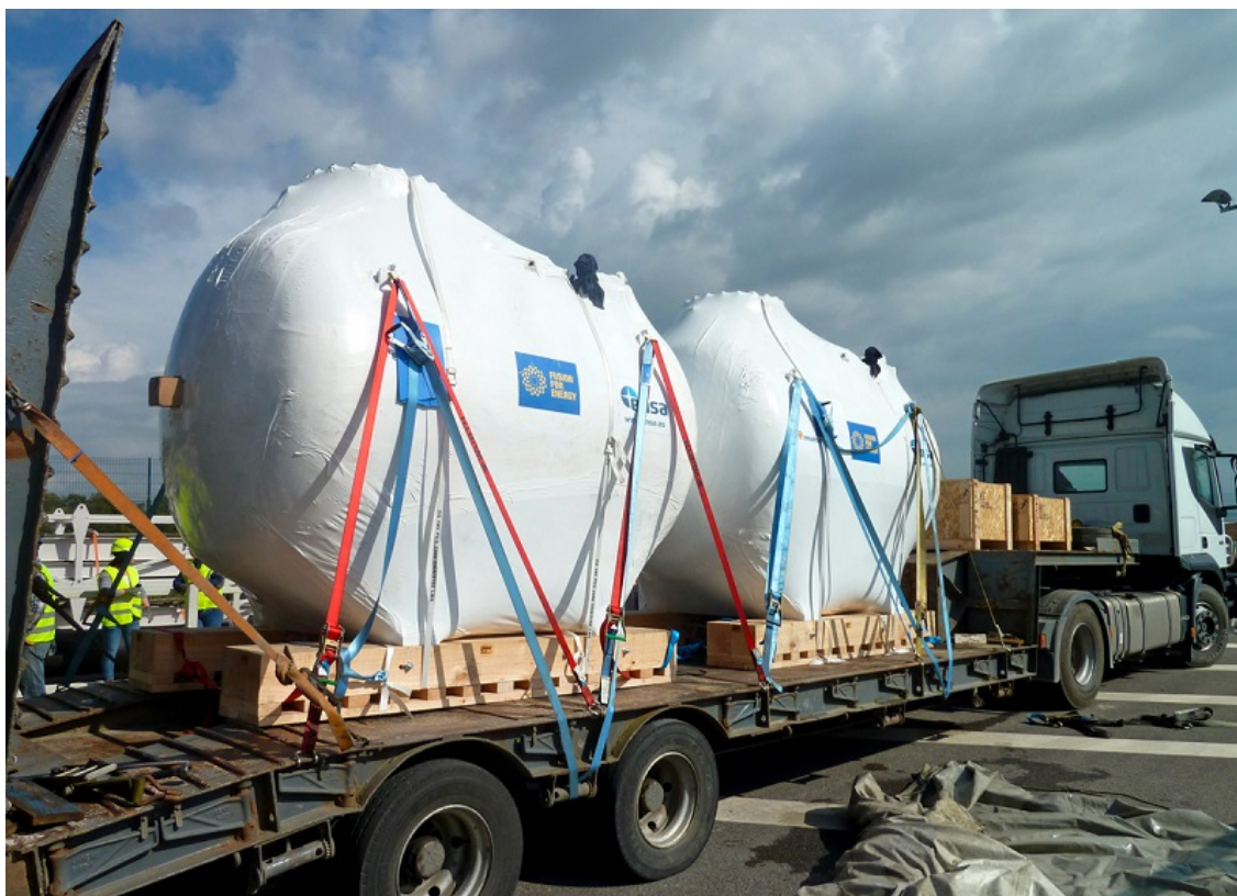
Figure 12: Two tritiated water holding tanks being delivered to Cadarache
