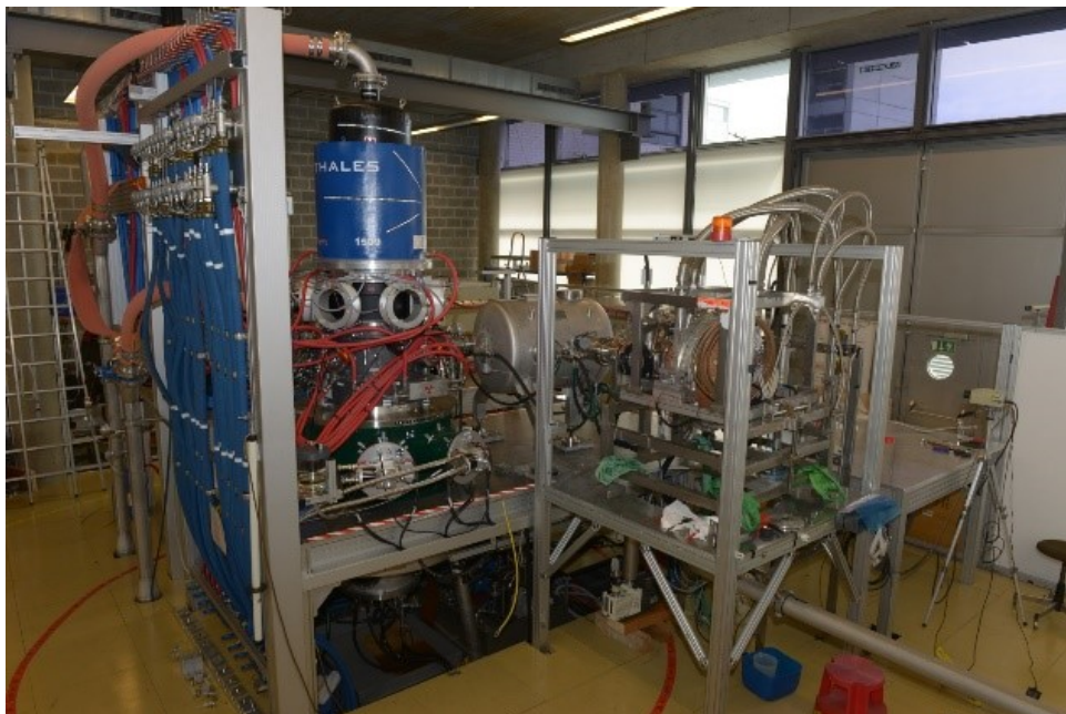
Figure 14: The prototype 1MW European gyrotron installed and undergoing testing in the new "Falcon" facility at the Swiss Plasma Center in Switzerland
