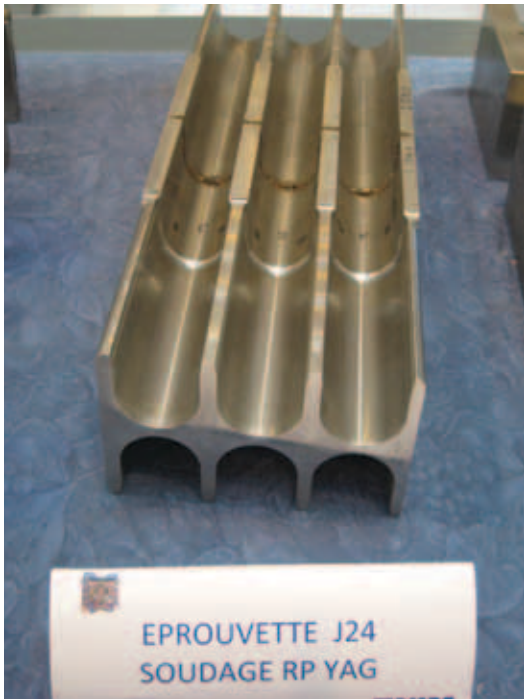
Welding mock-up by CNIM
