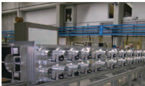
Aluminium mock-up in Legnaro, used to check the tunability of the RFQ
