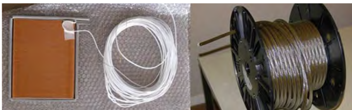
Fig. 19: First prototypes of magnetic sensors have been produced in 2010. These include the outer-vessel discrete coils (left) and continuous external Rogowski coil (which will be mounted inside several of the main TF coils)
