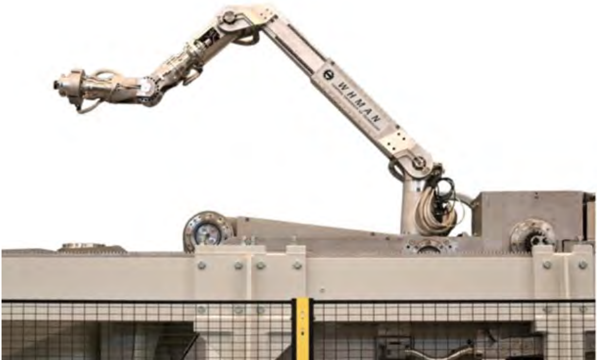
Fig. 10: Manipulator on board the CMM in DTP2 (courtesy of TEKES-VTT-IHA)
