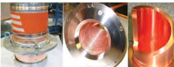
Fig. 17: Refurbished gyrotron prototype for ITER (from left to right): view of the coaxial gun (improved design), view of the beam tunnel internal structure designed to suppress parasitic oscillations, view of the upper part of the new high efficiency launcher.
