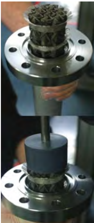
Fig. 14: Insertion of Sulzer packing into the cryo-distillation column (courtesy of KIT)
