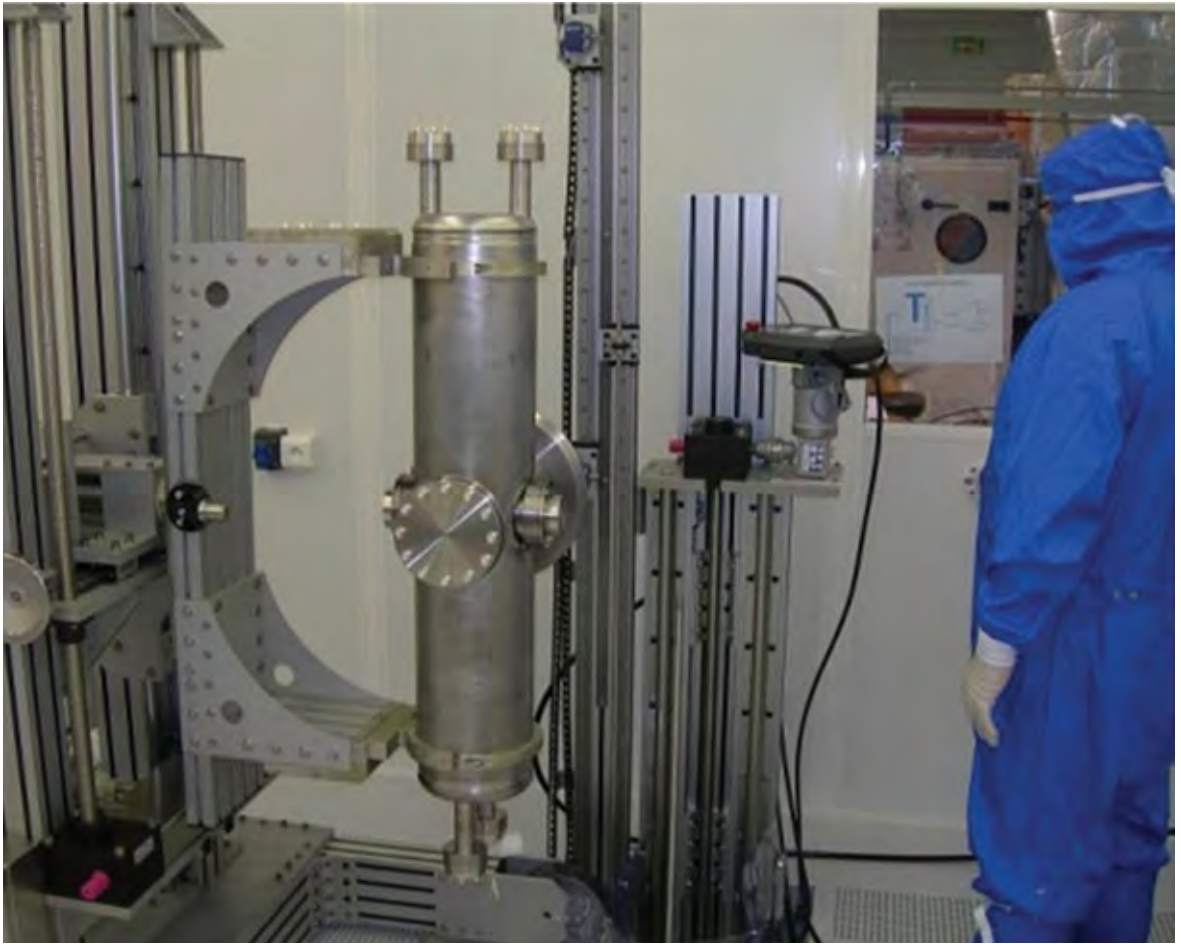
Fig. 30: High pressure rinsing of the Half-Wave Resonator prototype (P01) manufactured for the Superconducting RF Linac
