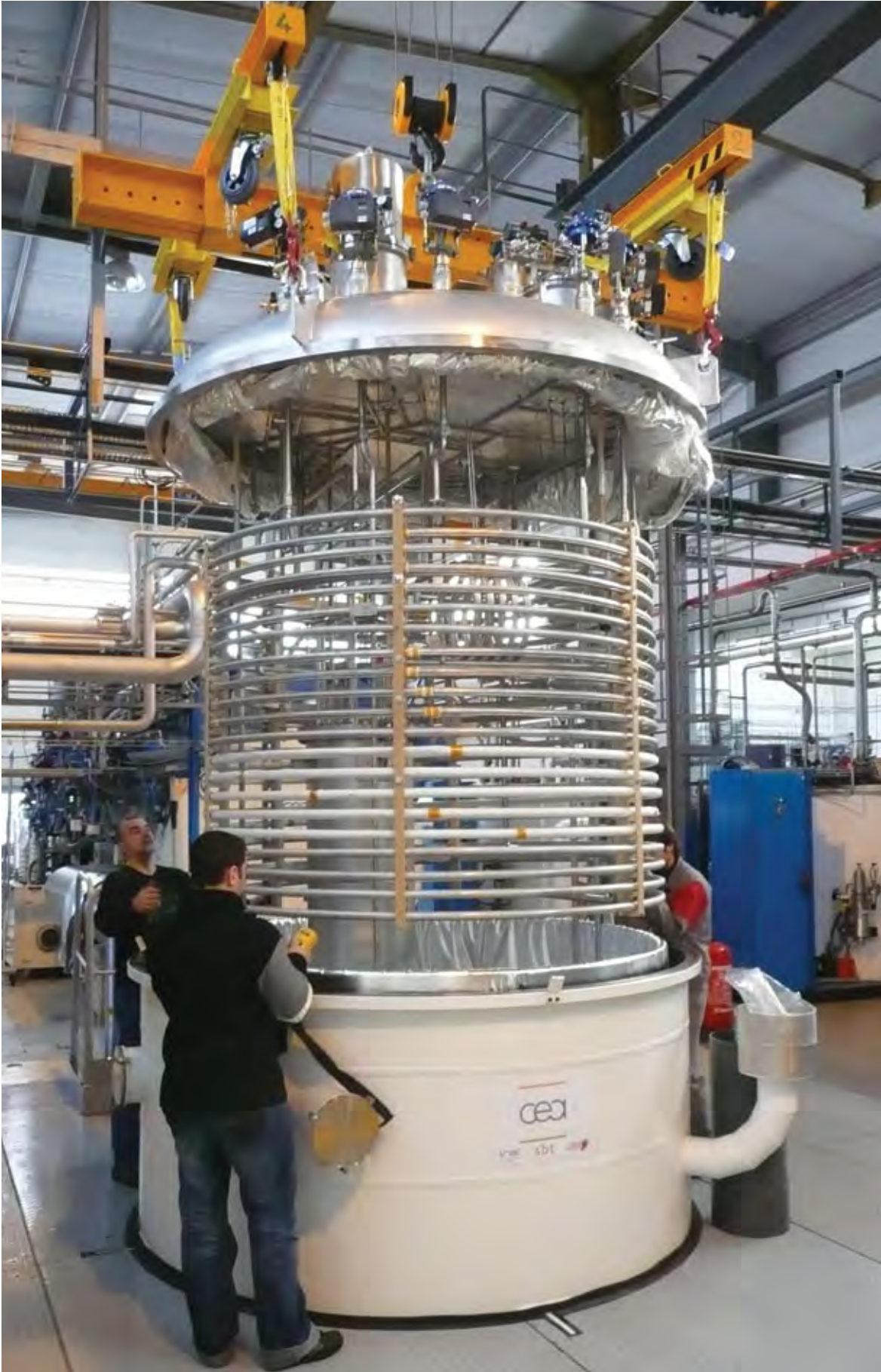
Fig. 27: The dedicated test loop HELIOS (courtesy of CEA / SBT Grenoble)
