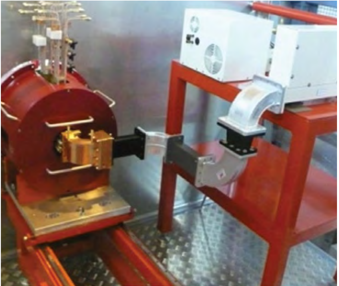
Fig. 28: Ion source and RF chain on HV platform
