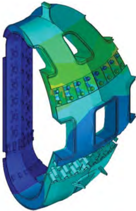
Fig. 24: Stress analysis of the Vacuum Vessel (left) and close-up (right)
