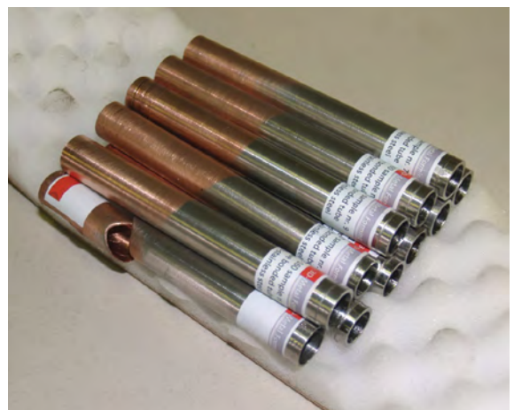
Explosion bonded CuCrZr to 316L pipe sections (3D metal forming BV, NL)
