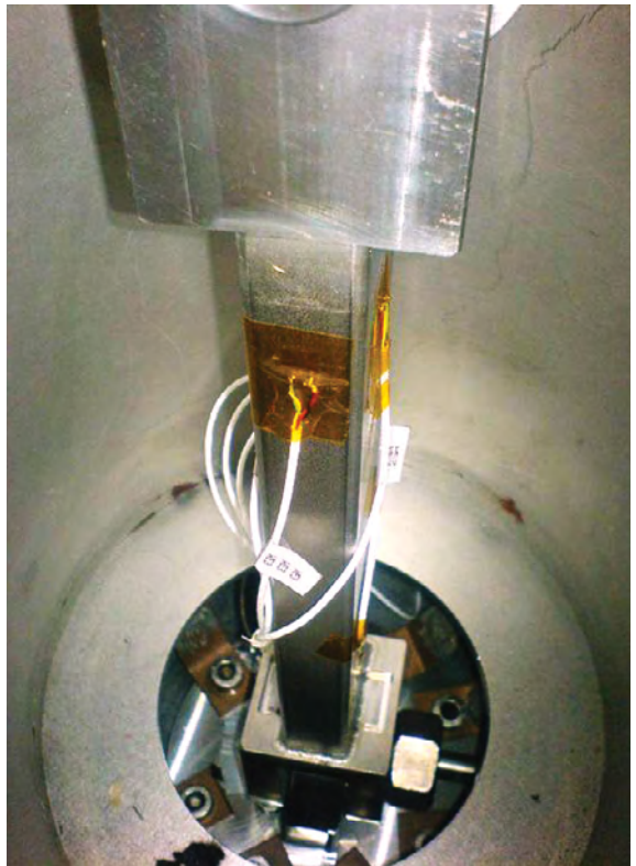
CEA Saclay - Friction tests of gravity supports
