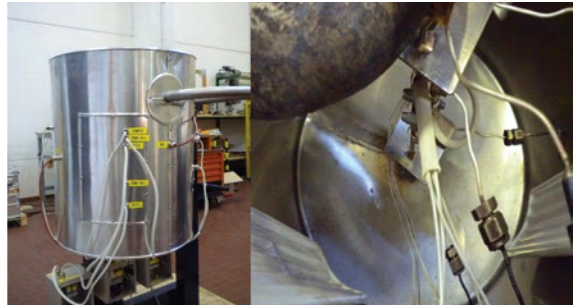
Mechanical assembly of the resistivity meter (left) and its sensor head (right)
