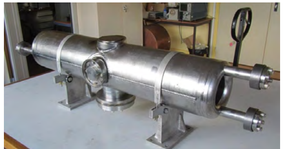
Repaired HWR cavity with the removal of the plunging system
