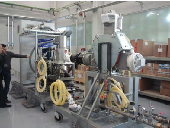
Prototype radio frequency module installed in the test facility
