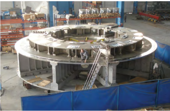
JT-60SA Cryostat base fully pre-assembled in factory in Spain, during final laser-tracker measurements
