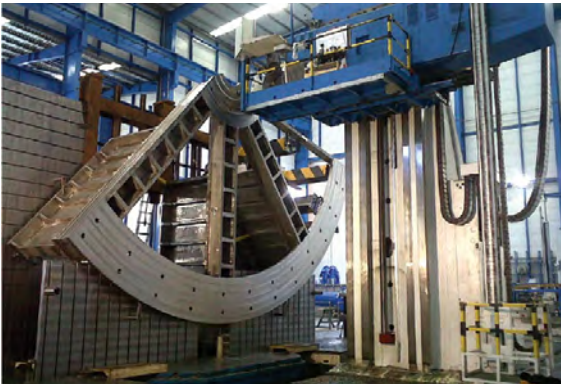
A lower sector of the JT-60SA cryostat base being machined by subcontractor ASTURFEITO
