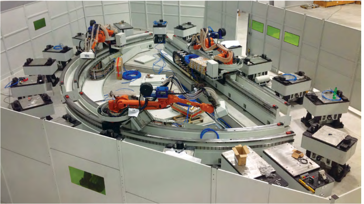
Cover plate laser welding station (courtesy of ASG)
