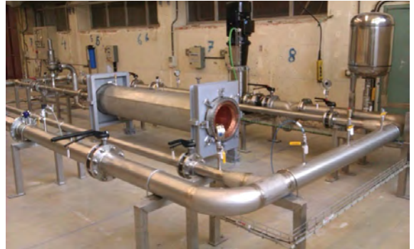
Hydraulic circuit for testing of the beam dump prototype
