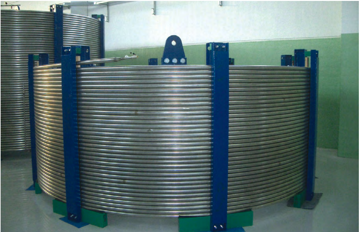
Conductor sDP1 at storage place ready for shipment (courtesy of ICAS)
