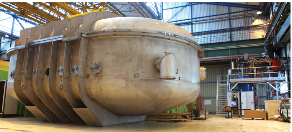
CEA Saclay - JT-60SA Toroidal Field Coil Cold Test Facility – Cryostat (Belgian contribution) positioned in the test hall
