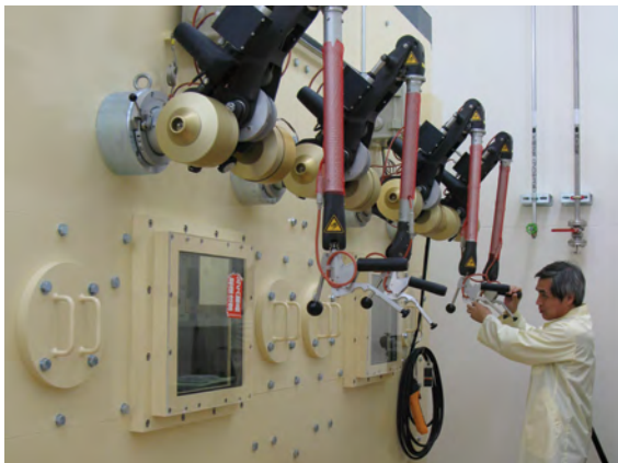
Manipulators in the materials test area of the DEMO materials laboratory
