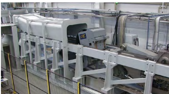
Concept prototypes and mock-ups of the ITER divertor remote handling system (DTP2 test facility)
