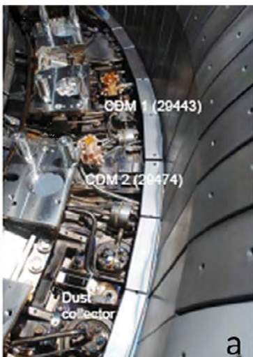
Capacitive diaphragm monitors (gauges for dust measurement) installed for testing in ASDEX UG
