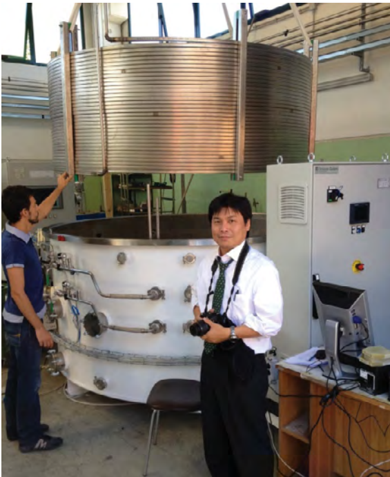
F4E - JTF-003 Pressure test / helium leak test at ICAS
