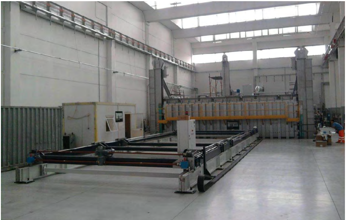
Heat treatment furnace and loading carriage (courtesy of ASG)
