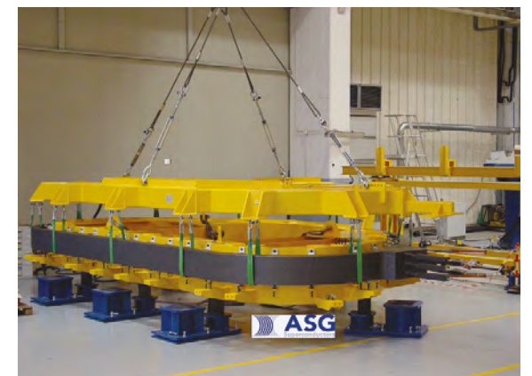
Winding Pack no. 1 (WP-01) placed on the tooling for case insertion at ASG
