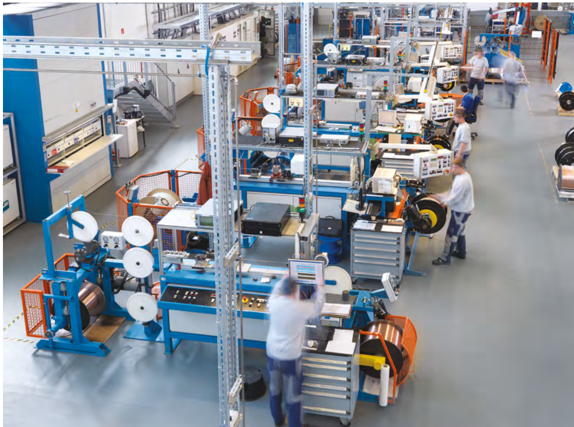
Final inspection on the Nb 3 Sn strand with an Eddy Current Test (courtesy of Bruker EAS GmbH)
