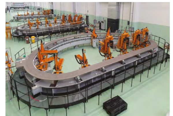
The three-turn insulation machines operating simultaneously on three different series production DPs (courtesy of CON)
