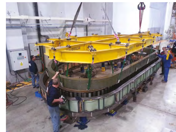
Coil no. 10 extraction from the impregnation mould at ALSTOM
