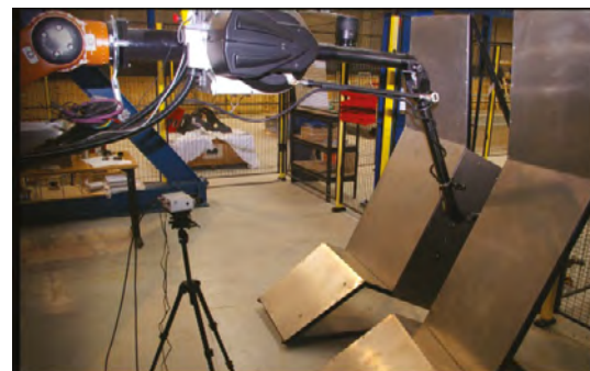
Master-slave tele-operation using a 3D stereo viewing system at OTL (OMF 272 contractor): the operator in the control room (left picture) is wearing 3-D glasses to watch the screen and control at distance the slave arm (right picture) located elsewhere (stereo-camera on the tripod)
