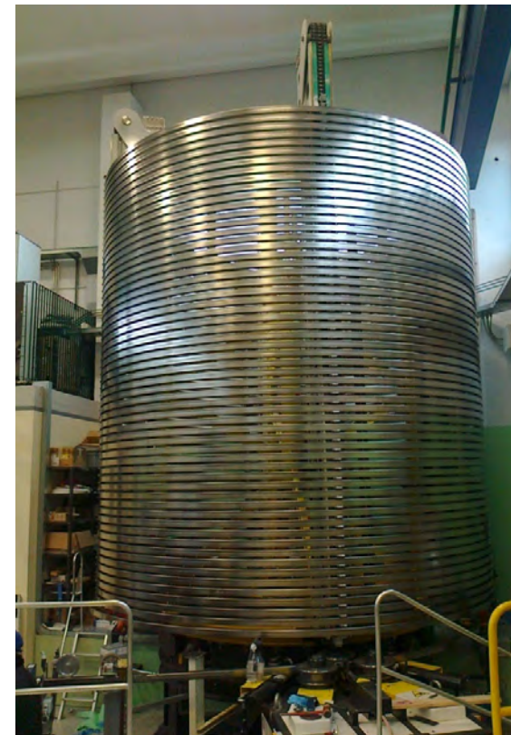
The second PF6 Poloidal Field production conductor length at the end of its spooling
