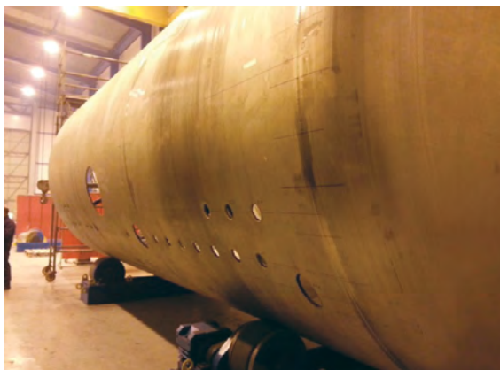
Shells of 100 m³ tank with holes for nozzles.
