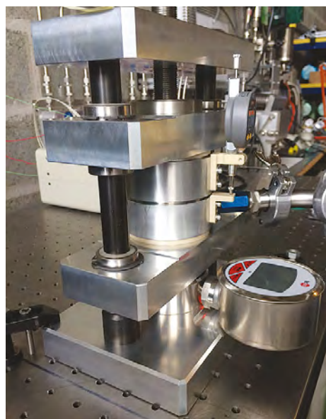
Test rig to characterise the mechanical behaviour of the double helicoflex seals and measure the leak tightness under axial loading and temperature variations
