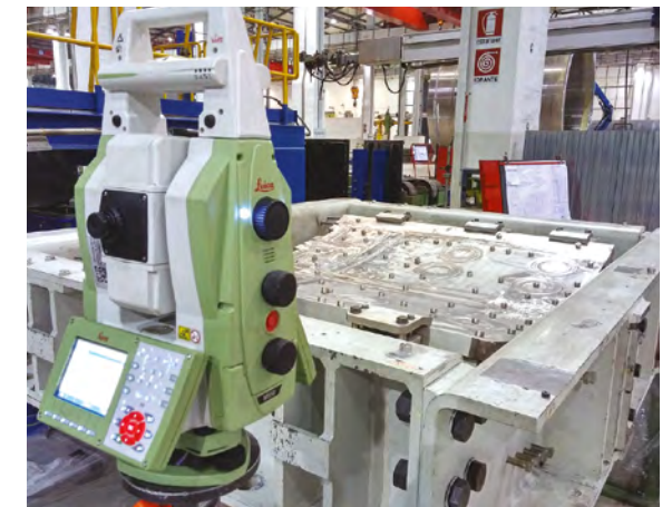
PS1 mock up under dimensional inspection.
