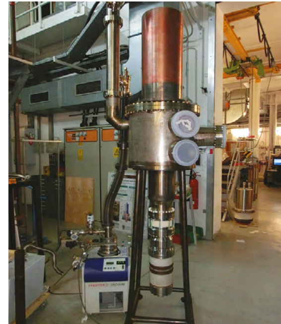
The 1 MW short pulse gyrotron assembled (F4E-OPE-458)
