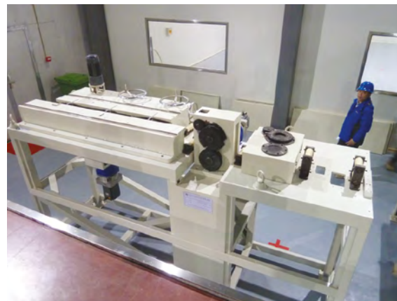
View of the Poloidal Field PF6 winding tooling line straightening unit – during commissioning at ASIPP
