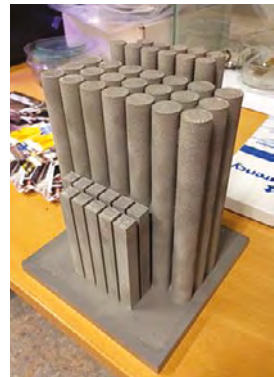
Figure: Sample material made out of austenitic stainless steel by additive manufacturing by Mid-Sweden University, Sweden, to be characterised by Tecnalia, Spain
