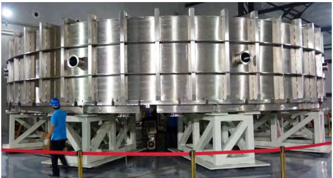
Some of the developments carried out at the ASIPP facility in Hefei, China and its suppliers: View of the PF6 DP Vacuum Chamber during commissioning at ASIPP
