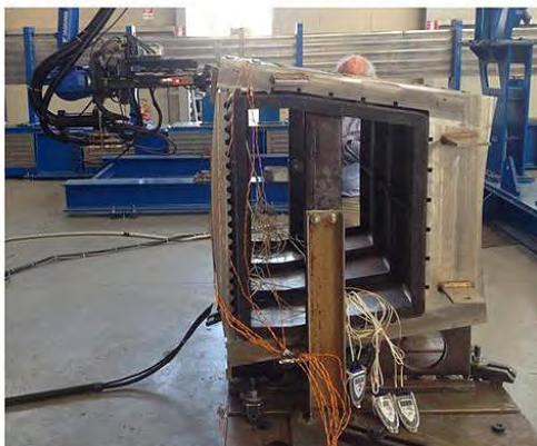
Welding distortion analysis: One metre long and full-scale TF coil case cross section mock-up completed in September
