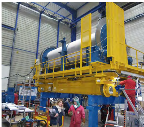
One of the trolleys of the 750 t North crane during the assembly phase at the factory
