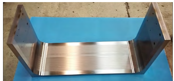
Half-size mock-up of TBM first wall realised with standardised welding procedure specifications (ATMOSTAT, CEA), after removal of the canister and machining; final tolerances are within specifications.
