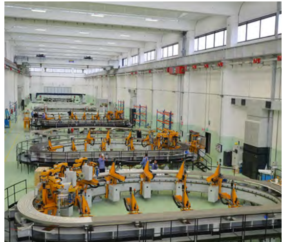
Three turn insulation machines, operating simultaneously on three different series production DPs in ASG, La Spezia
