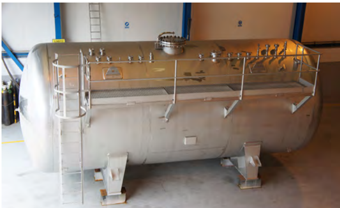
100 m 3 tank at manufacturer before Factory Acceptance Tests
