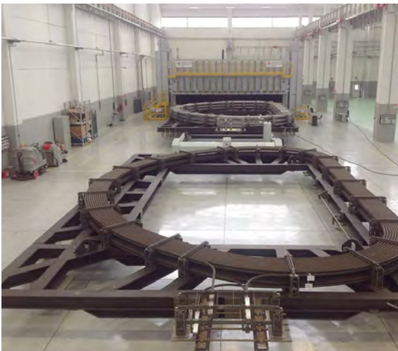
At the oven entrance, three series production DPs on their frame, being loaded to start the heat treatment. At the front, two previously treated DPs in ASG, La Spezia
