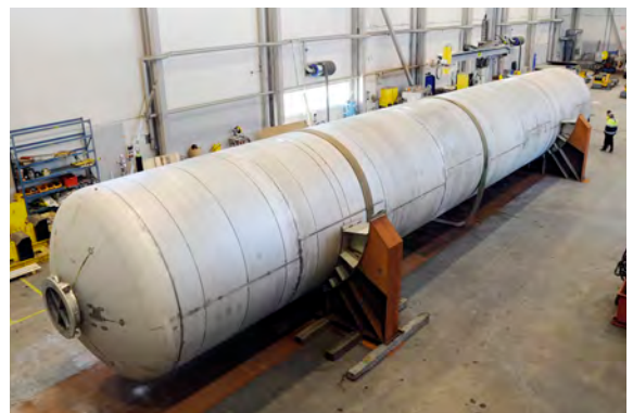
LHe tank inner vessel helium leak test
