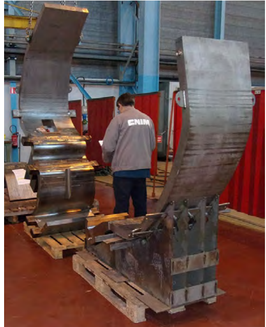
Cassette body prototype under fabrication at CNIM
