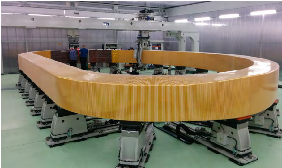
Automated Winding Pack ground insulation operation in ASG, La Spezia (Courtesy of ASG)
