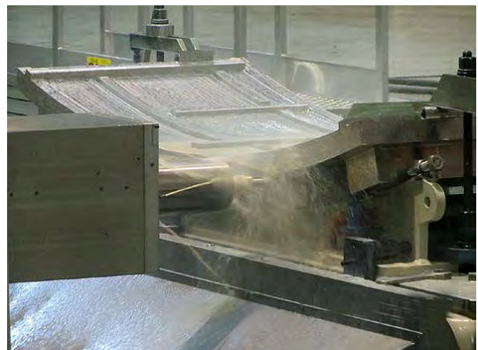
Machining activity on large forging
