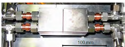
Installation of the irradiated Be mock-ups in JUDITH-1
