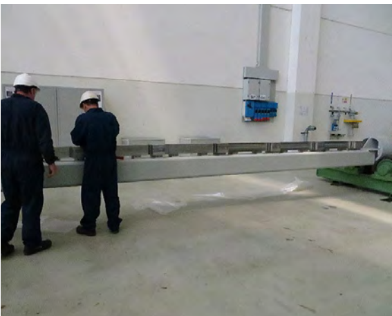
First weld of vacuum vessel sector 5 - Central rib of the poloidal segment 1
