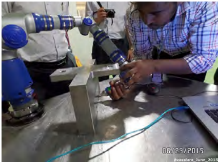
A vacuum vessel shielding block inspection
