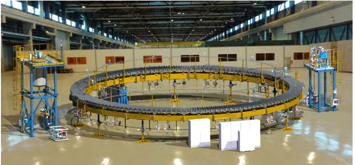
PF 2-5 DP impregnation system – system overview
