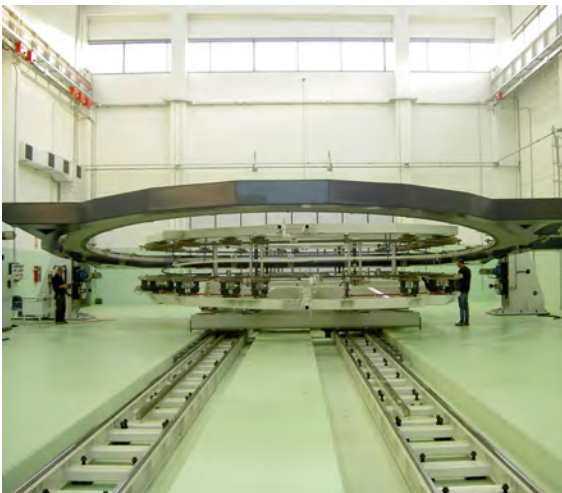
Insertion of a DP inside the Radial Plate grooves in ASG, La Spezia. (Courtesy of ASG)
