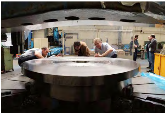
The pump plug of the pre-production cryopump in manufacturing
