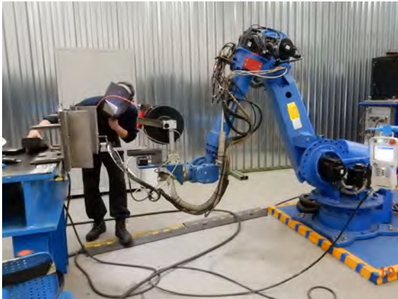
Automatic TIG welding qualification
