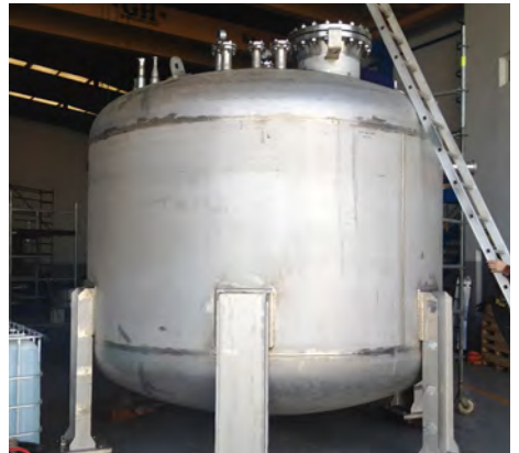
20 m 3 tank before Factory Acceptance Tests
