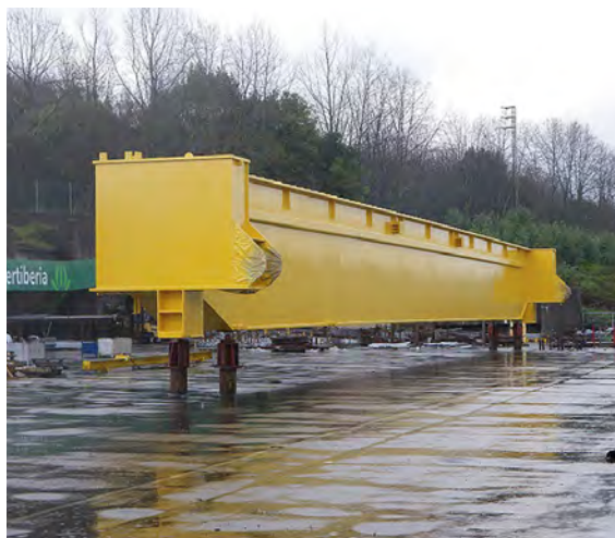
Crane 750 t first girder, stored at the factory location before assembly and squaring
