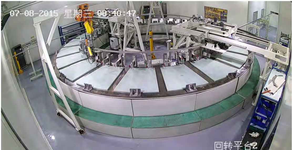
Some of the developments carried out at the ASIPP facility in Hefei, China and its suppliers: View of the Poloidal Field PF6 winding tooling machine in commissioning
