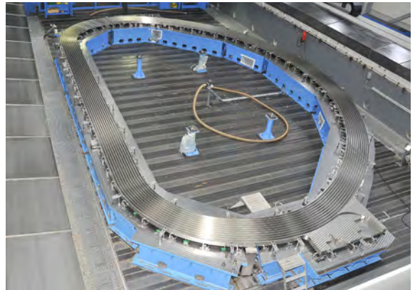
Machined Radial Plate at the CNIM site (Courtesy of CNIM)
