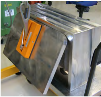
Closure of side caps onto the first wall for the realisation of a TBM box one-third mock-up (ATMOSTAT)
