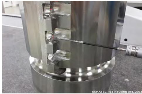
A flexible housing CMM inspection
