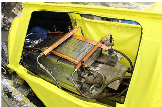
First Wall semi-prototype manufactured by the Consortium IBERDROLA/Amec FW/Leading and tested at JUDITH-2
