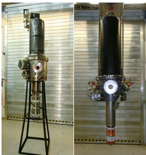
The short pulse (left) and the CW (right) EU gyrotron prototypes
