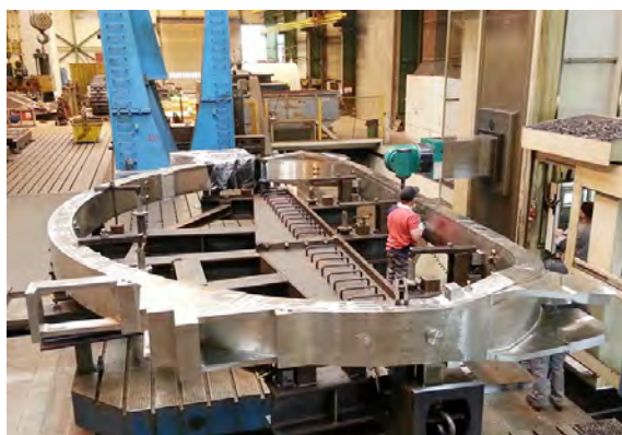
Final machining of coil no. 10 (November 2015) (Courtesy ALSTOM/CEA).
