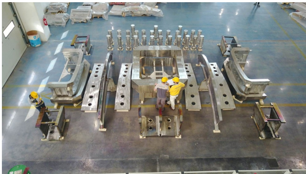
Figure 2: Assembly work underway on one of the sub-segments of the fifth Vacuum Vessel sector
