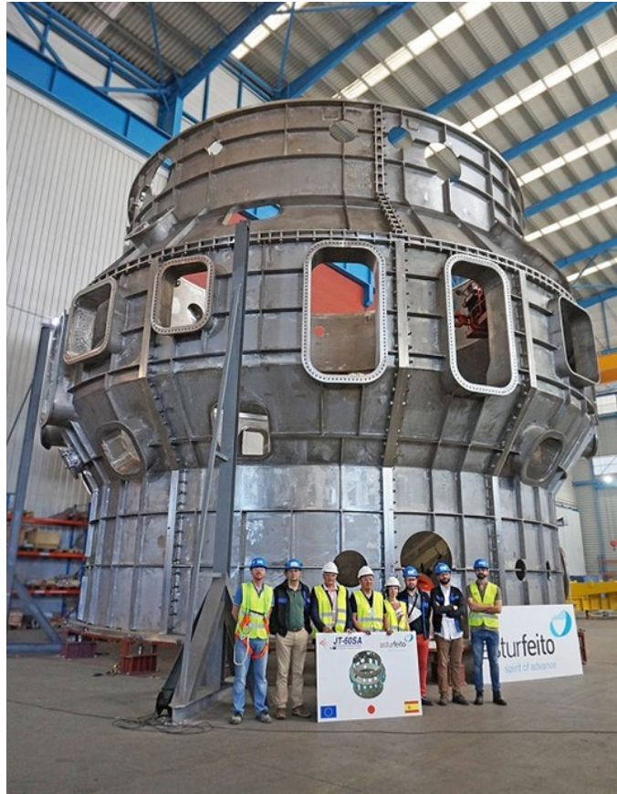
Figure 16: The completed JT-60SA cryostat vessel body with representatives of F4E, CIEMAT and Asturfeito S.A. prior to its shipping to Japan
