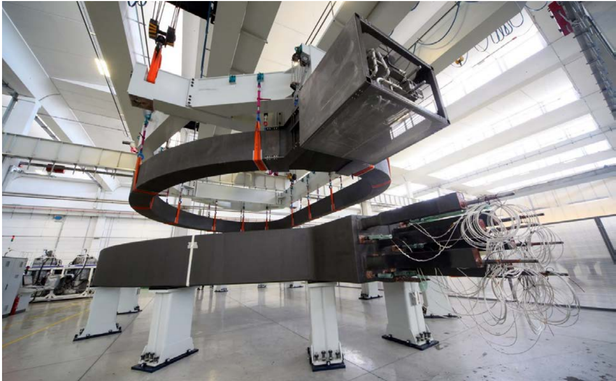
Figure 4: The first two Winding Packs for the superconducting Toroidal Field coils
