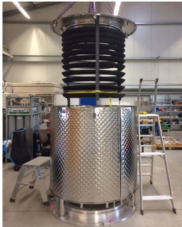
Figure 11: Assembly of the Pre-Production Cryopump prior to shipping to ITER
