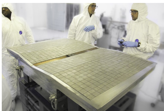
Figure 7: Assembly of the beryllium tiles on the first wall panel full-scale prototype
