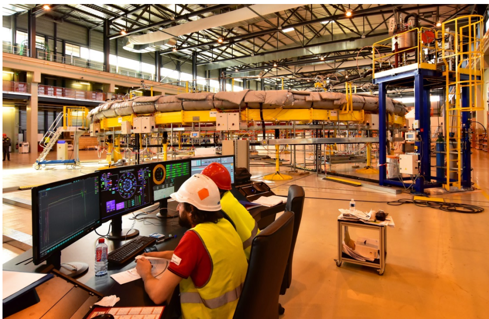
Figure 5: Dummy Poloidal Field Magnet Double Pancake (PF5) undergoing Vacuum Pressure Impregnation in F4E's PF Coil Fabrication Facility, Cadarache, France)
