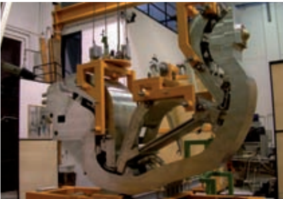
Image 2 Integrated Divertor Cassette (Courtesy ENEA)
