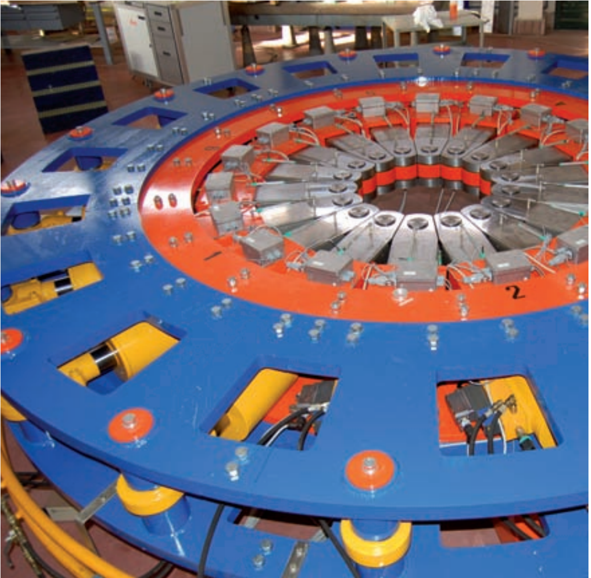
Image 1 Magnets: Tests on sub-scale pre-compression ring (Courtesy ENEA)
