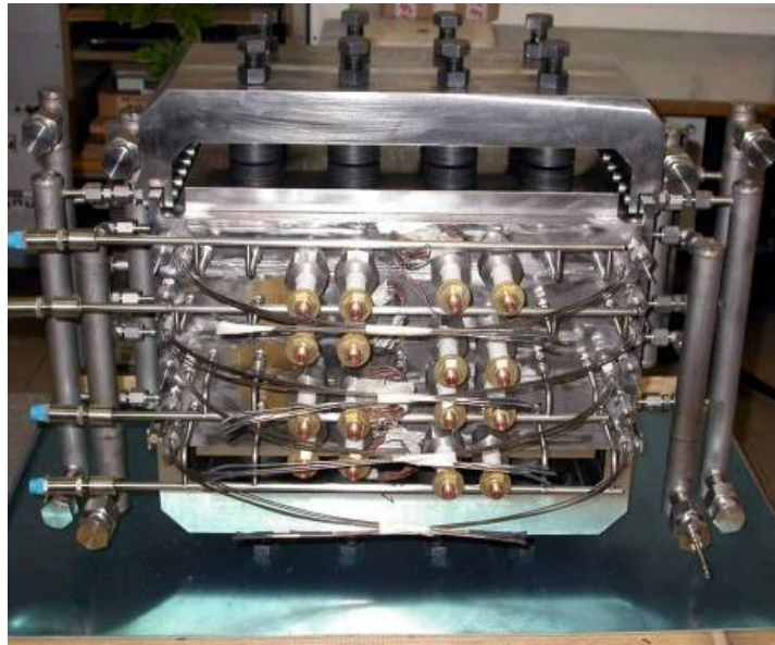
Figure 52 – External view of the HEXCALIBER mock-up containing piled-up layers (not visible) of lithium ceramic / beryllium pebbles and cooling plates for investigation of thermo-mechanical behavior of the HCPB TBM.
