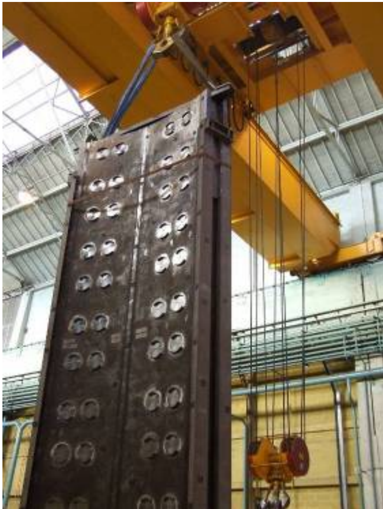
Figure 20 - Electron Beam Welded Sector Mock-up
