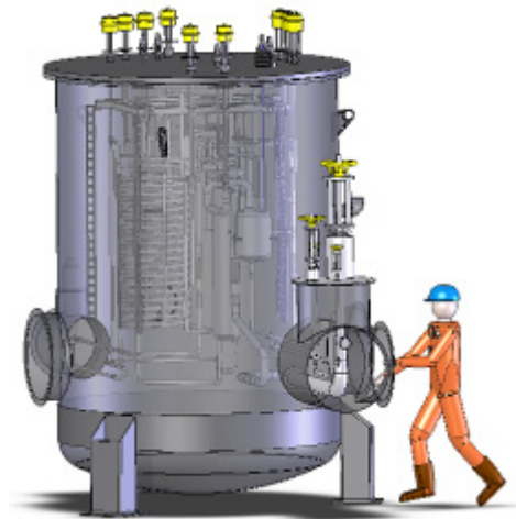
Figure 33 - Artists impression of the proposed cryostat for the cryogenic test loop
