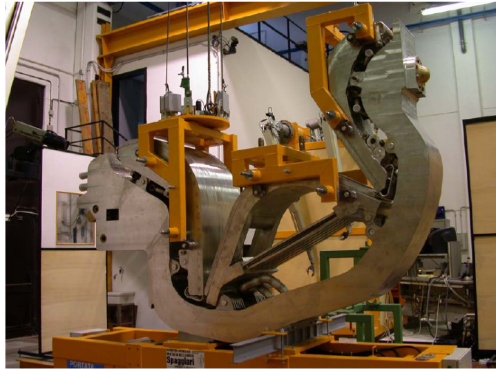
Figure 25 - Integrated divertor cassette
