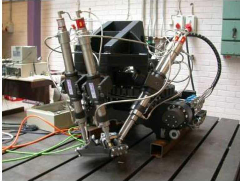
Figure 21 - Sector Welding Robot
