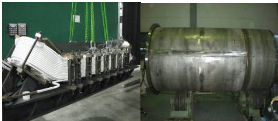
Figure 57 - EDIPO dummy coil after reaction heat treatment (left) and its containment steel cylinder 35 mm thick (right)
