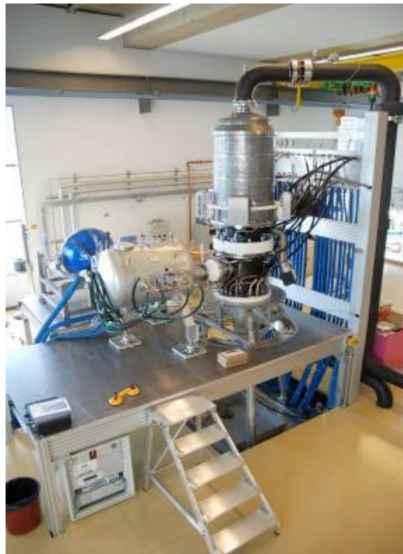
Figure 38 - EC Test Facility in CRPP-Lausanne and gyrotron under test
