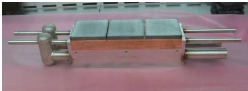
Figure 23 - EU FW Qualification mock-up after test at NRI
