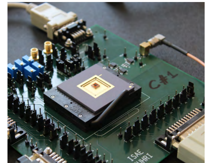
Image sensor mock-up on the test board part of the FURHIS project (Fusion for Energy Radiation hard Imaging System) signed between F4E and OTL
