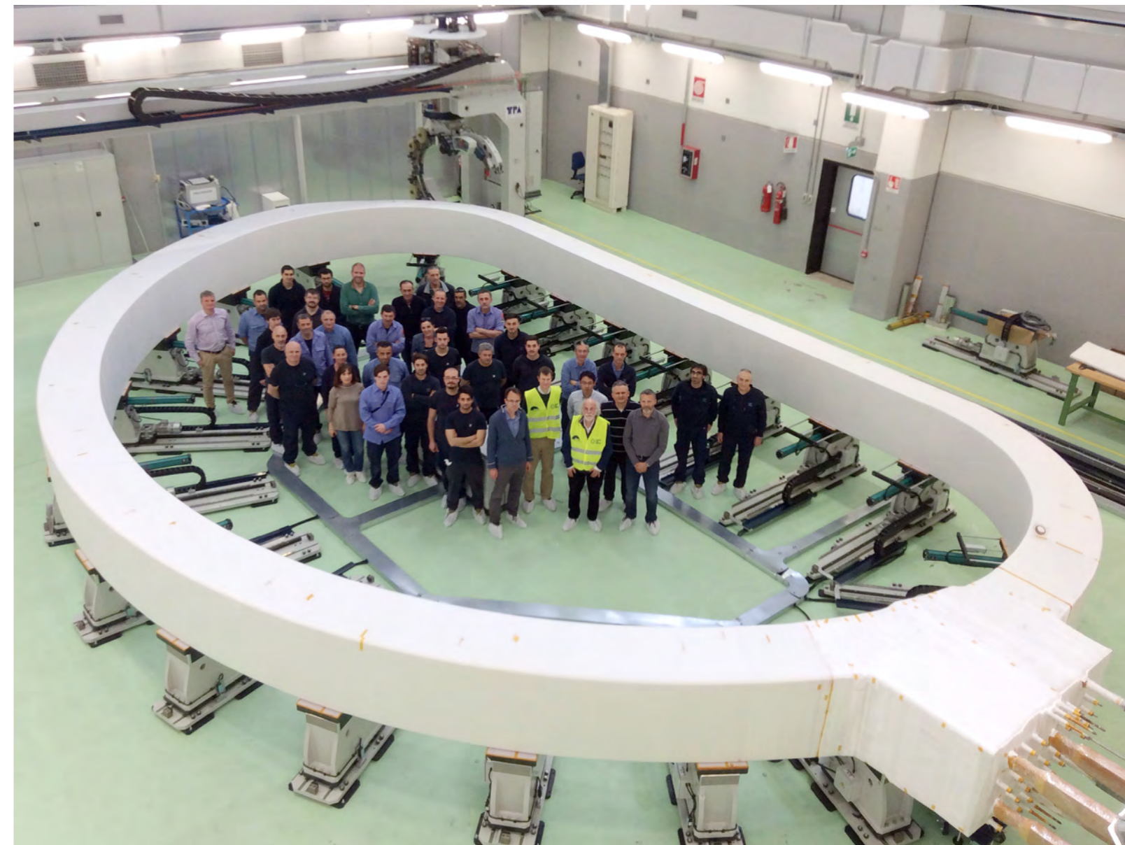
Representatives of F4E, ITER IO and F4E contractors standing inside the first ITER Toroidal Field coil winding pack - one of the biggest magnets to be manufactured.
