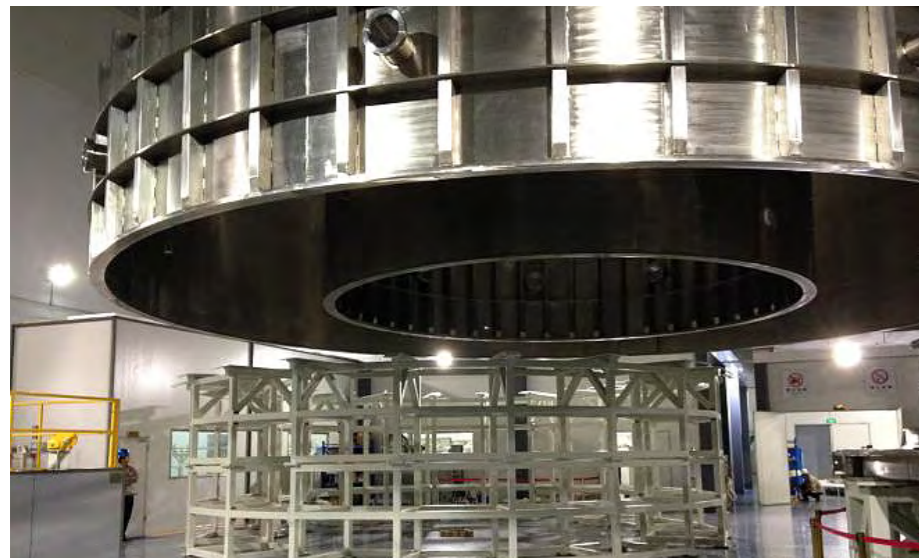
Placing the lead of the leak test chamber on the metallic structure in order to check that it can support a heavy load
