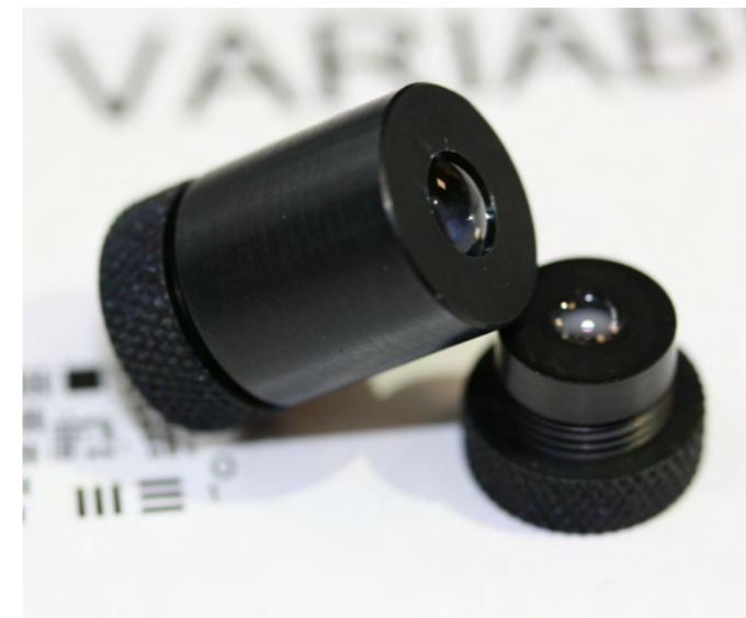
Mock-up of the optical subsystem part of the FURHIS project (Fusion for Energy Radiation hard Imaging System) signed between F4E and OTL
