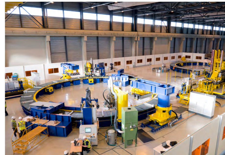
View of the Poloidal Fields coils facility with some first equipment installed for the production of the ITER coils
