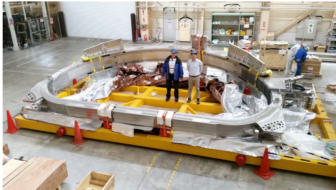
F4E's Technical Officers A. Cardella & L. Novello stand by the first JT-60SA TF coil in Japan
