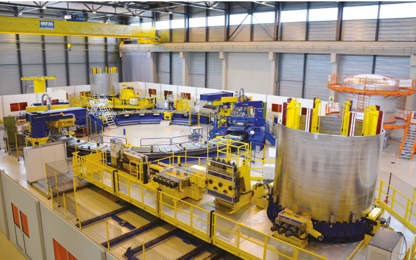
Winding tooling to be used for the manufacturing of ITER Poloidal Field coils, PF coils Facility, Cadarache, October 2016.
