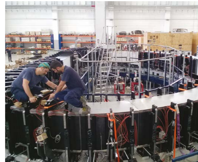
The inner-core of the Toroidal Field coil covered with resin pads, ASG Facility
