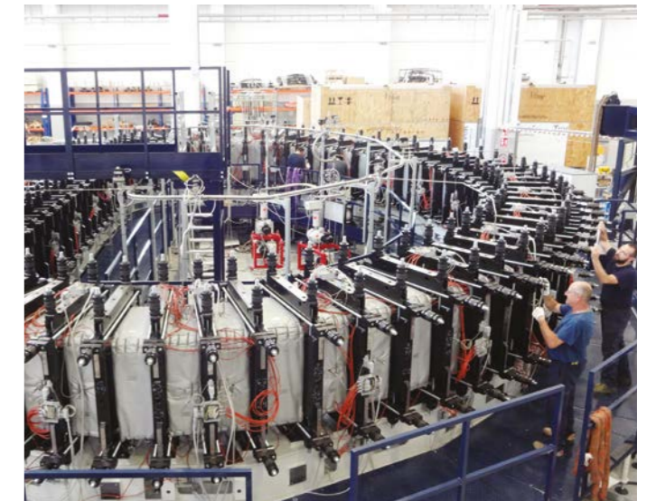
Compacting the inner-core of the first Toroidal Field coil, ASG Facility
