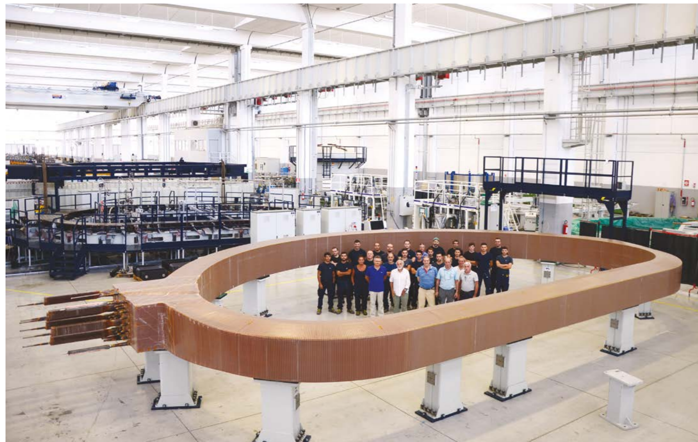
First impregnated winding pack, the core of an ITER Toroidal Field coil, ASG Facility, La Spezia, Italy
