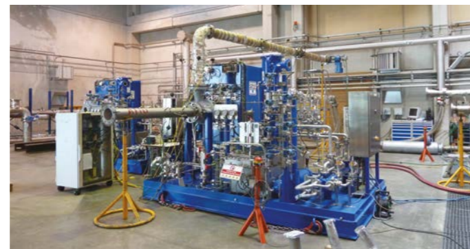
Turbo booster turbine able to generate 500 KW of cooling power fully assembled for testing, Cryostar (France)
