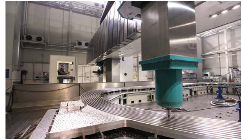
Tool machining the grooves of a radial plate
