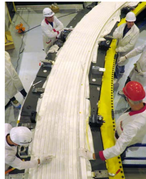
Team of technicians checking the manufacturing of the insulated dummy conductor, ITER Poloidal Field coils Facility, Cadarache, November 2016
