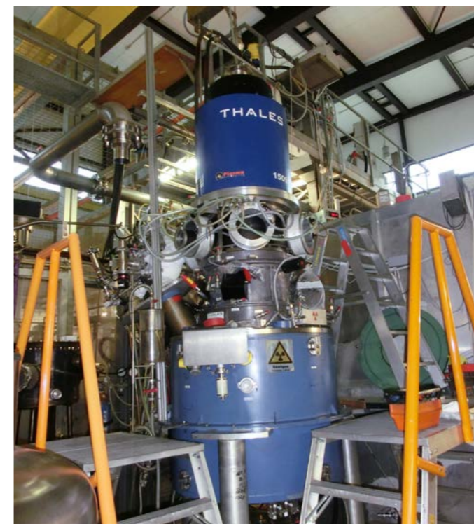
The 1 MW gyrotron prototype manufactured in Europe by French company TED on behalf of F4E
