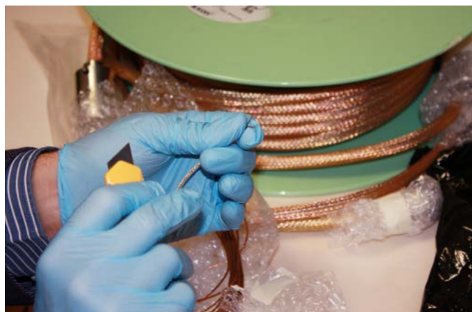
One of the Continuous External Rogowski (CER) coils undergoing acceptance testing earlier this week at the ITER site
