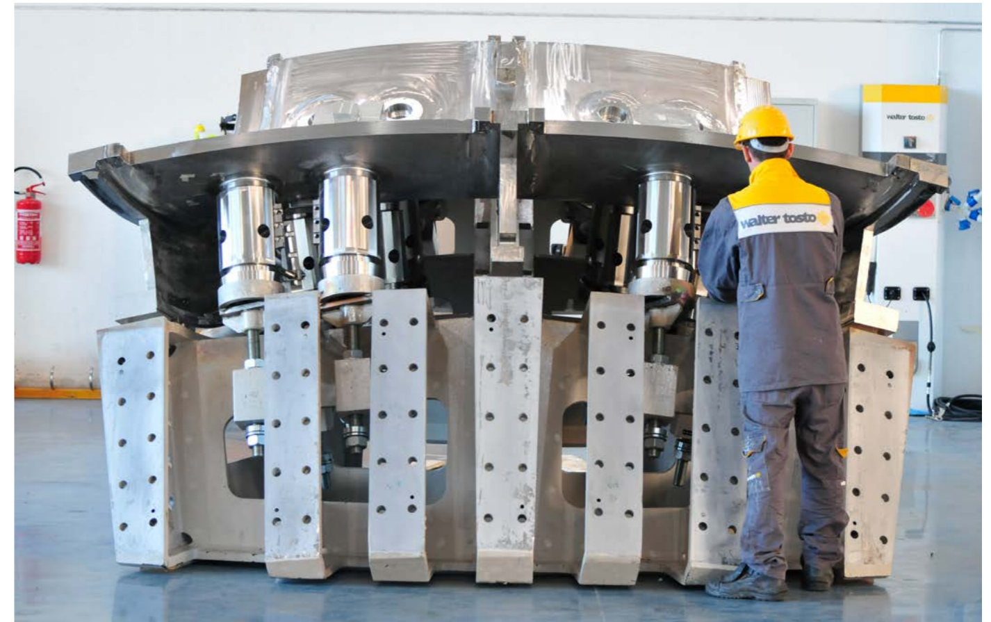
For the first time, smaller parts of a poloidal segment have been welded together to form a bigger piece (Image courtesy of Walter Tosto)
