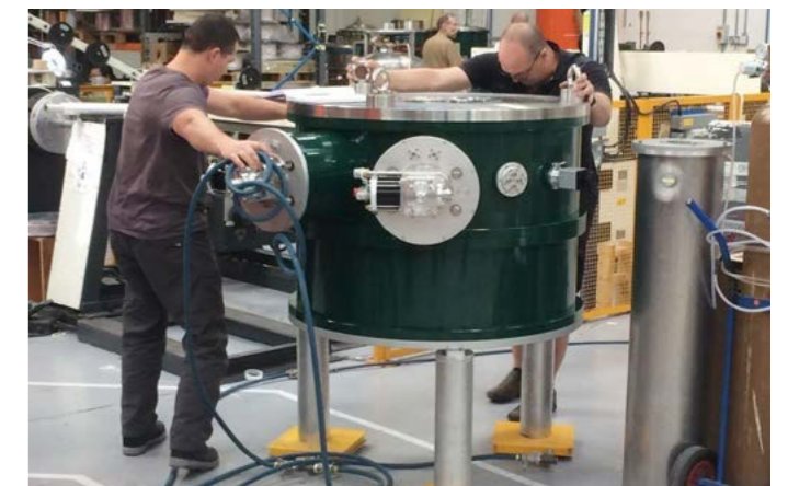
The magnet which will be joined to the gyrotron prototype and tested at SPC.
