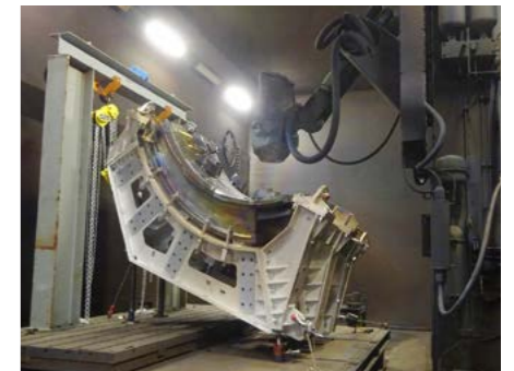
The sub-assembly in the vacuum chamber ready for electron beam welding of flexible housings
