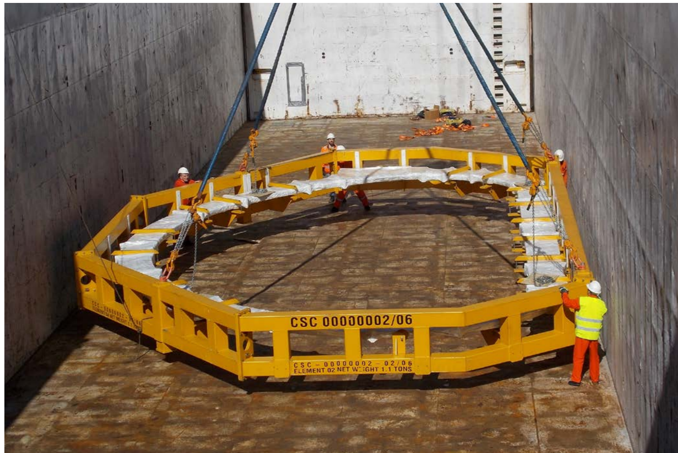
The final radial plate manufactured by SIMIC is loaded on the vessel
