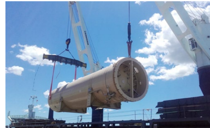
Unloading the liquid nitrogen tank (LN2) at the industrial port of Marseille, May 2017 © DAHER
