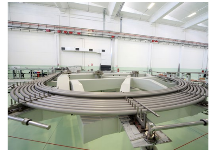
Winding the final conductor for Europe's ITER Toroidal coils, ASG Superconductors, La Spezia, Italy
