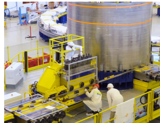
CNIM technicians supervising the manufacturing of the European Poloidal Field coils in F4E’s Facility, Cadarache
