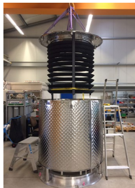
Assembly of the cryopump at Research Instruments, Germany © F4E
