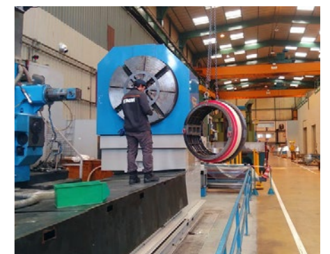
Installing the Pre-Compression Ring prototype in order to perform checks © CNIM
