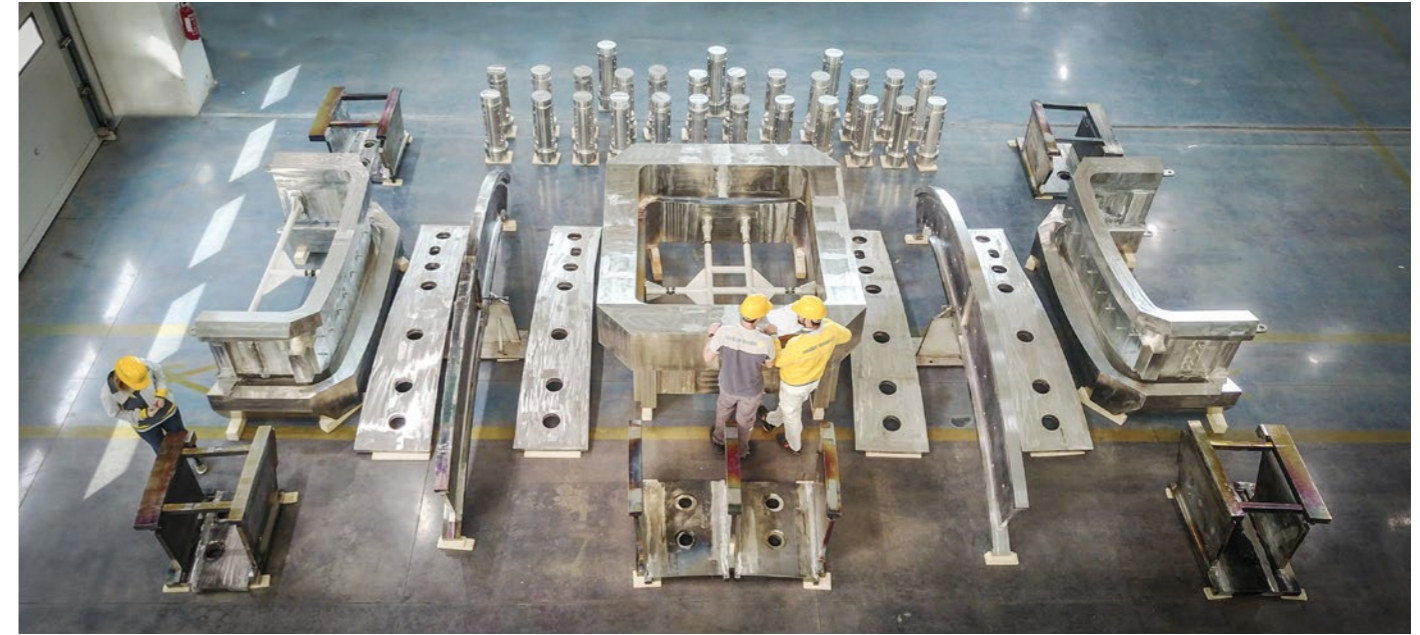
Parts placed together before assembly of the segment PS3 for the first VV sector, sector 5, at Walter Tosto
