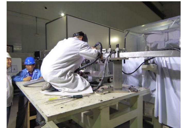
Working on the joint terminations of one Double Pancake of Poloidal Field coil 6, ASIPP, China
