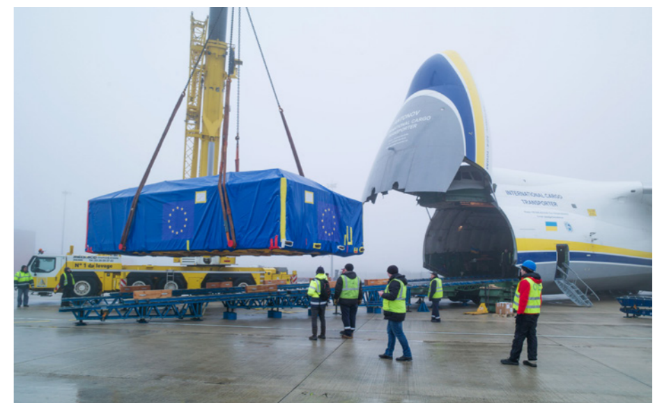
Loading of the last JT-60SA TF coils on to the plane bound for Japan.
