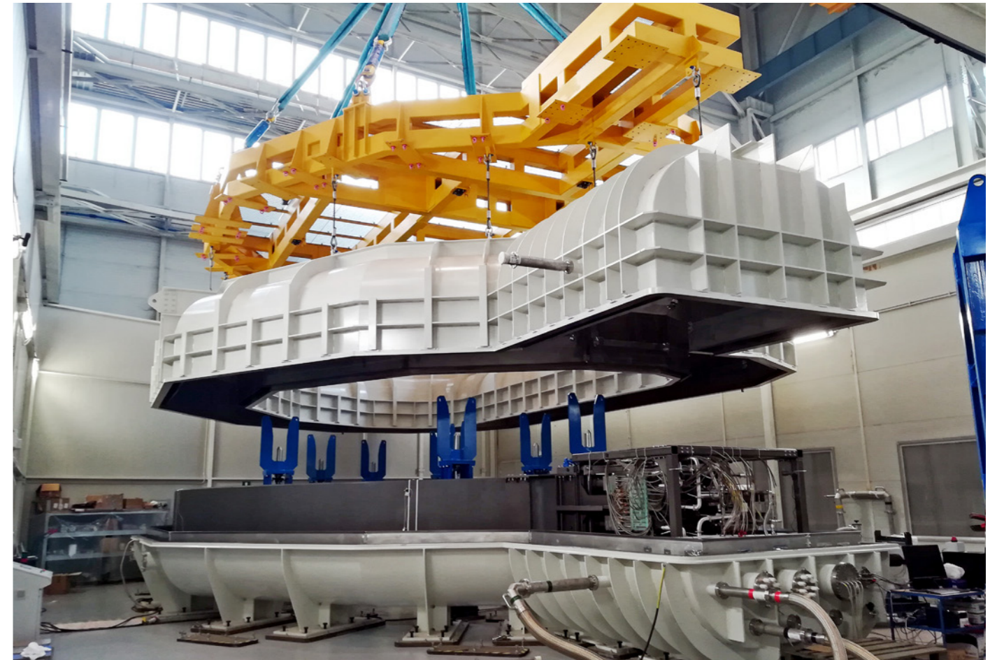
Europe's first Toroidal Field coil winding pack to undergo cold tests, SIMIC, port of Marghera, Italy © SIMIC
