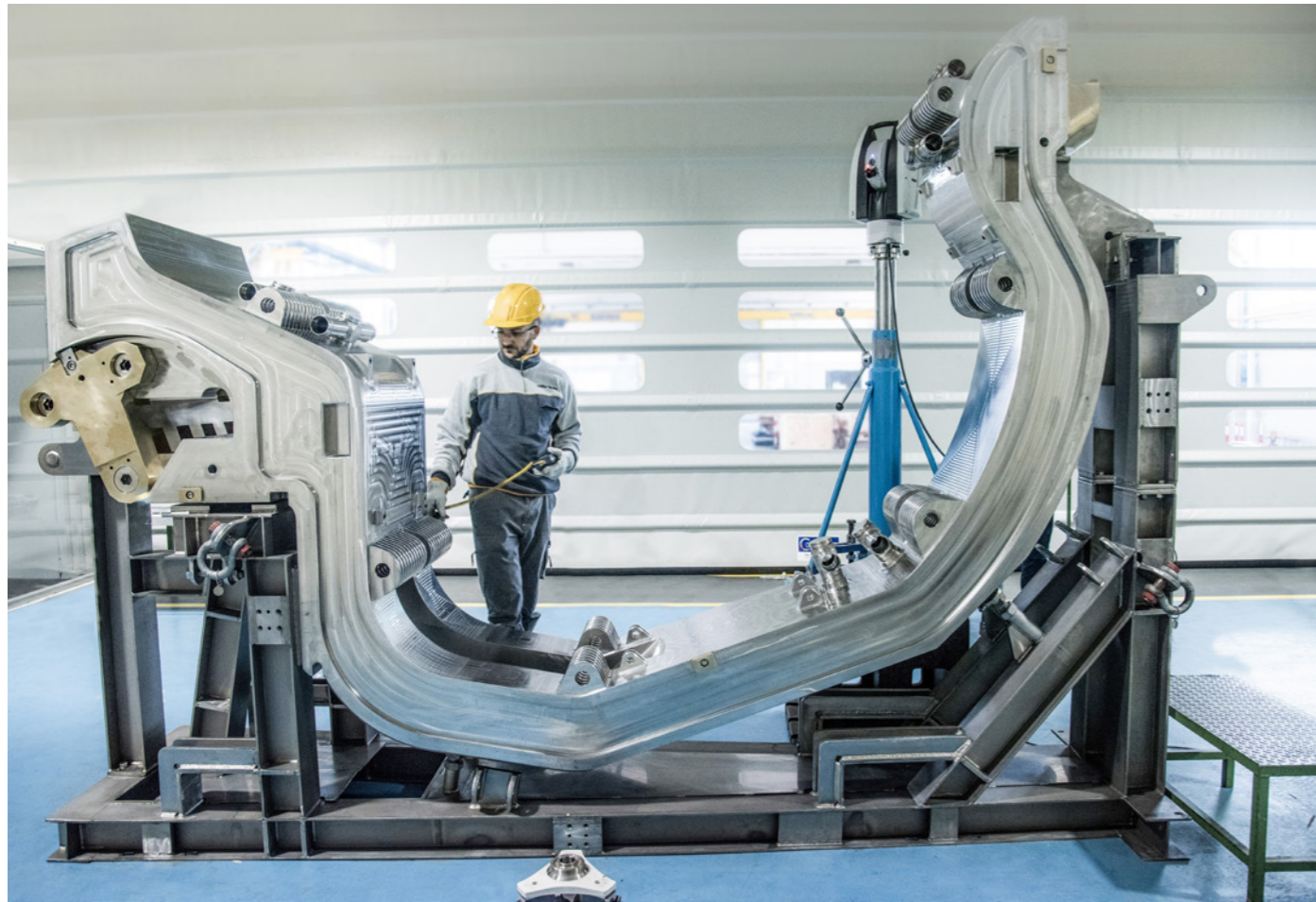
European real-size prototype of ITER Divertor Cassette manufactured by Walter Tosto © Walter Tosto
