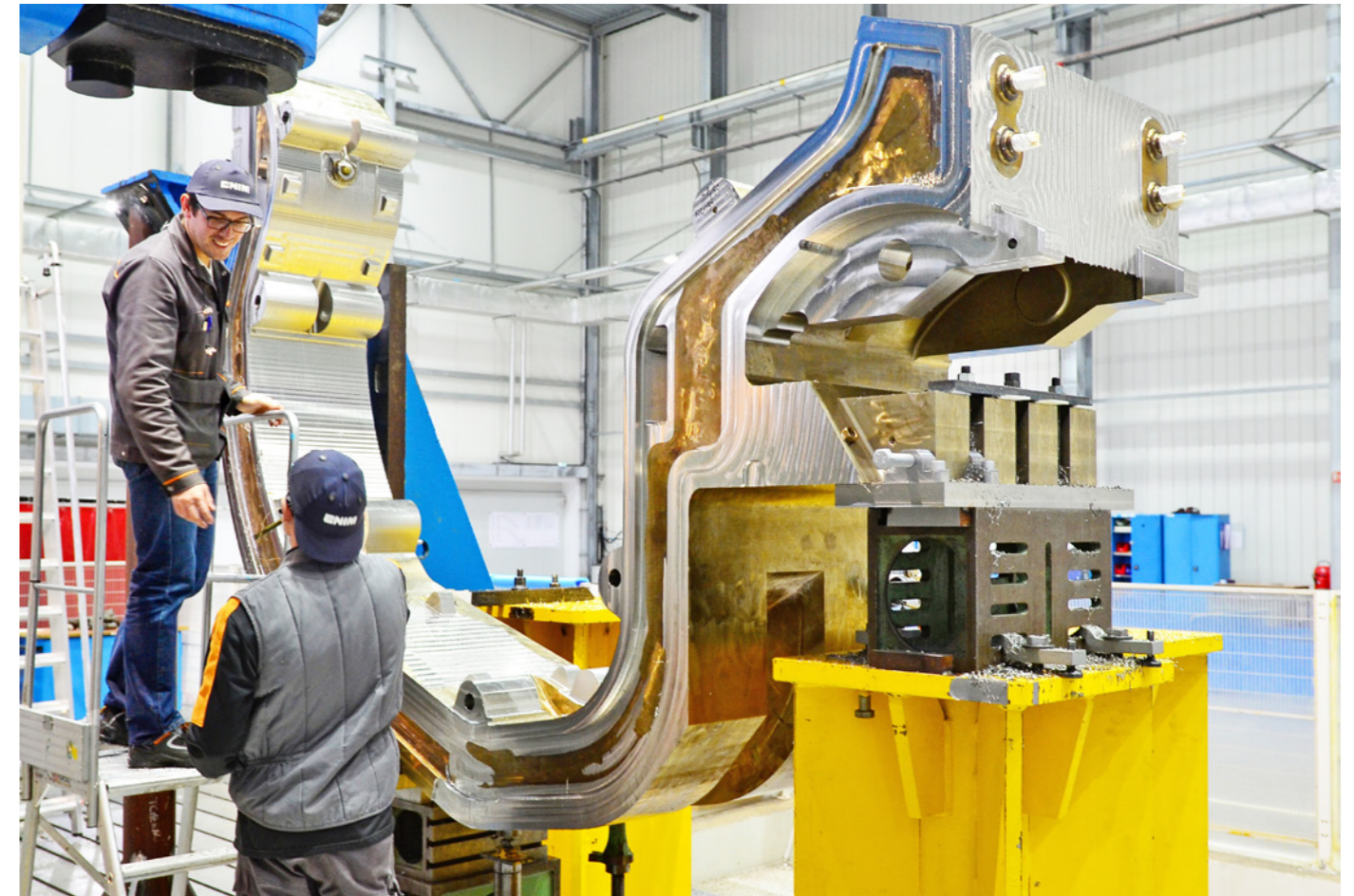
European real-size prototype of ITER Divertor Cassette manufactured by CNIM-SIMIC © CNIM
