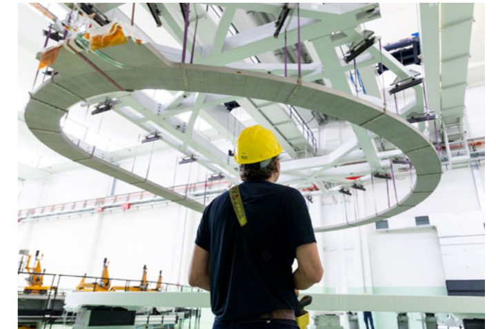
Technician lifting a Double Pancake to position it on another station, ASG Superconductors, La Spezia (Italy) © Andrea Botto
