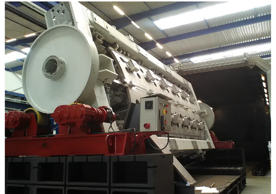
Three sub-assemblies manufactured by Mangiarotti (for sectors 5 and 4) and Ensa for sector 3) are being electron-beam welded at Pro-beam.
