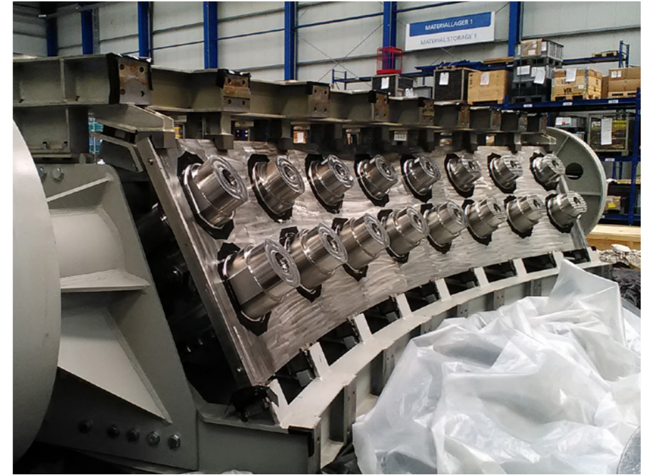
A sub-assembly manufactured by Mangiarotti for the Vacuum Vessel ready for electron-beam welding at Pro-beam.
