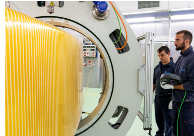
Technicians carrying out ground insulation on a Winding Pack, ASG Superconductors, La Spezia (Italy) © Andrea Botto
