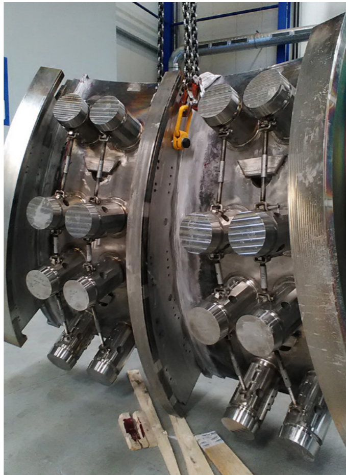
A sub-assembly of a sub-assembly segment for sector 4, manufactured by Walter Tosto and welded at Pro-beam.
