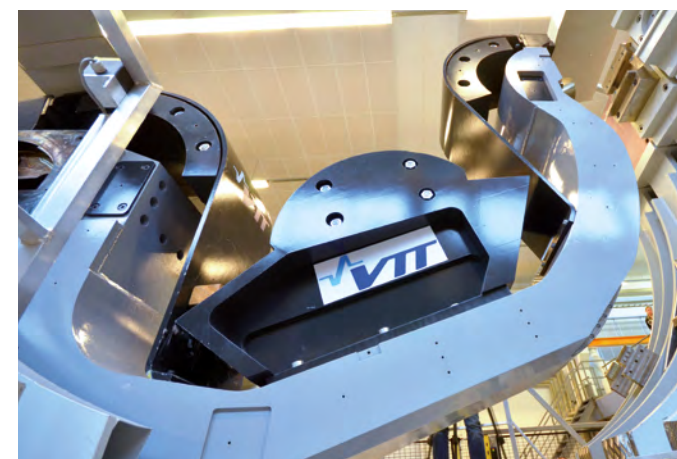
The ITER divertor cassette mock-up. Its weight is 10 tonnes and measures 3.3 m x 2.3 m x 0.8 m.
