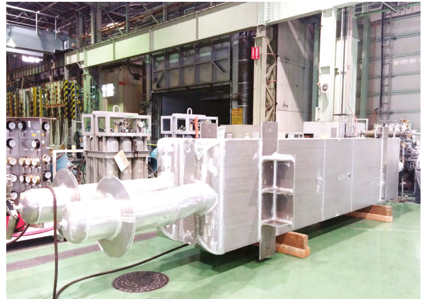
The brazed aluminium heat exchanger for the LN2 Plant at the workshop of Sumitomo Precision Products
