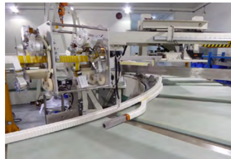
From top to bottom and left to right: Technicians carrying out manually the insulation of the joggle, PF6 Coil Manufacturing Workshop; Insulation winding tooling, PF6 Coil Manufacturing Workshop; Vacuum chamber to perform leak tests, PF6 Coil Manufacturing Workshop, ASIPP China.
