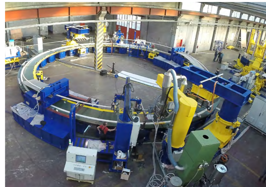
The Poloidal Field coils winding tooling table, SEA ALP workshop, Turin (Italy).
