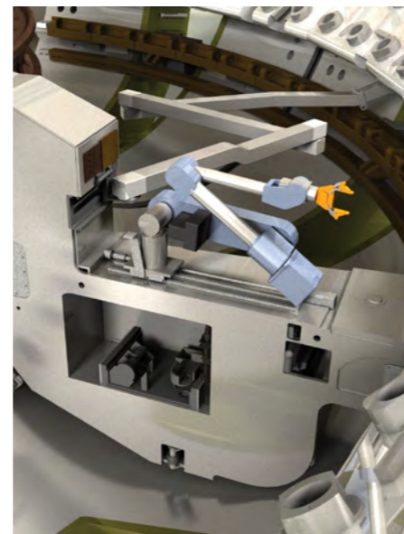
3D image of the remote handling system for ITER divertor – Photo credit: Assystem
