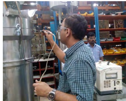
Technician inspecting the valve that will control the helium flow from the 80K loop boxes to the thermal shields and cryopumps of the ITER machine, manufactured by Flowserve, India.
