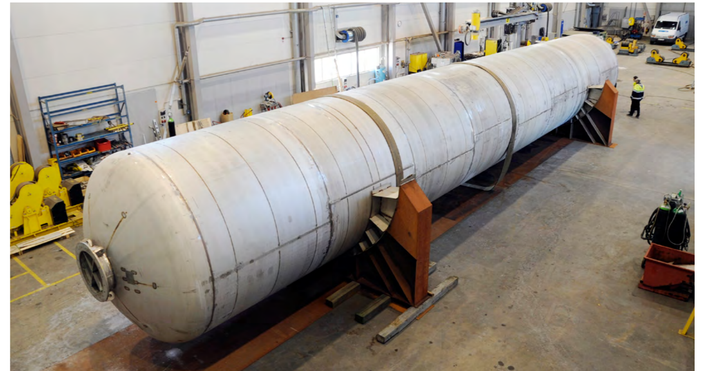
The liquid helium inner-tank, designed and manufactured by CryoAB, part of the contract signed between Air Liquide Global and EC Solutions and F4E.
