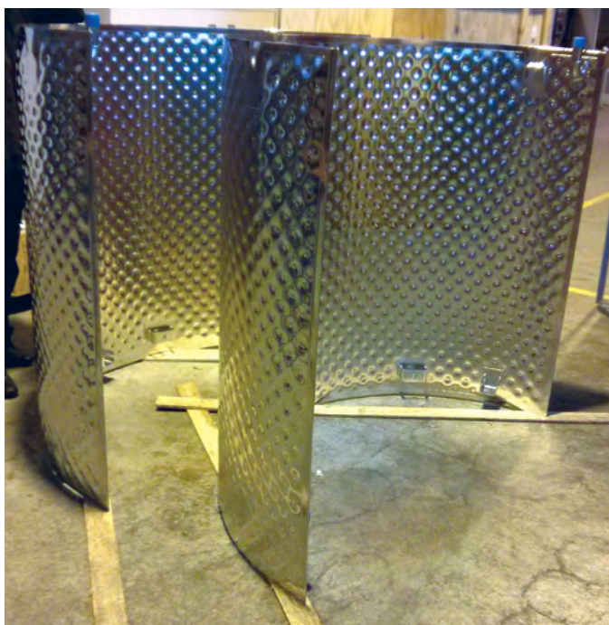
Manufactured hydroformed components of the PPC thermal shields Copyright SDMS/Ziemex
