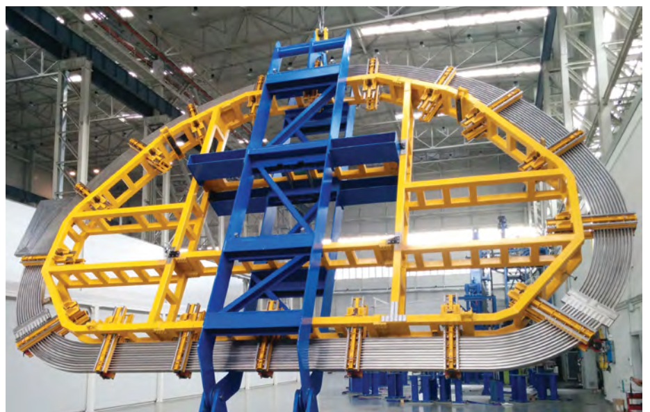
Overview of the SIMIC facility in Italy, Porto Marghera, while works of radial plate tilting are being carried out
