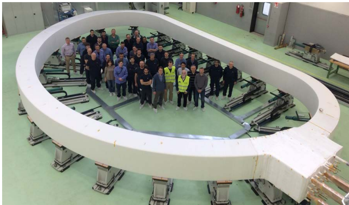
Figure 2: The first-ever Winding Pack for the Toroidal Field coils, completion of which met a major ITER Council milestone (ASG Superconductors, La Spezia, Italy)
