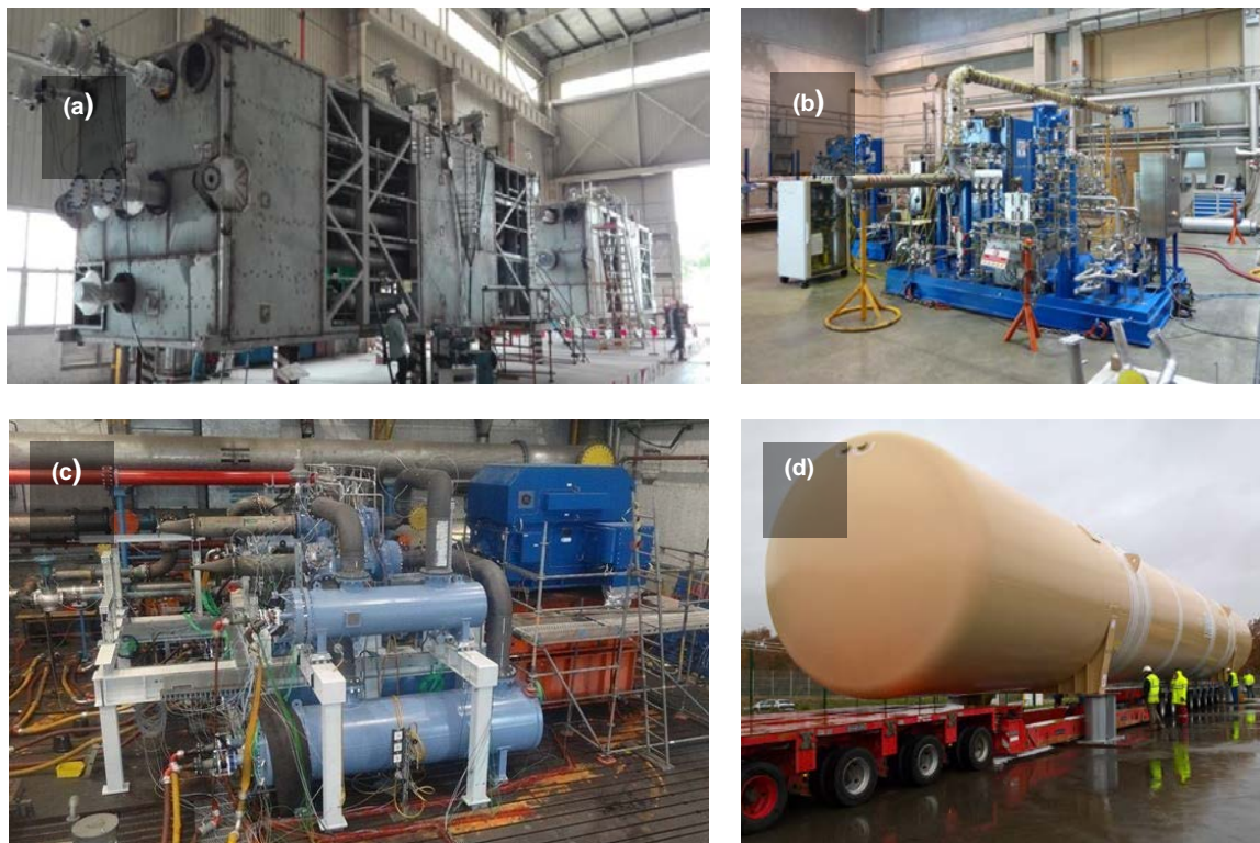
Figure 4: Components of the ITER cryogenic cooling systems manufactured by European industries under contract with ITER (a) cold boxes, (b) turbine, (c) compressor and (d) quench tanks
