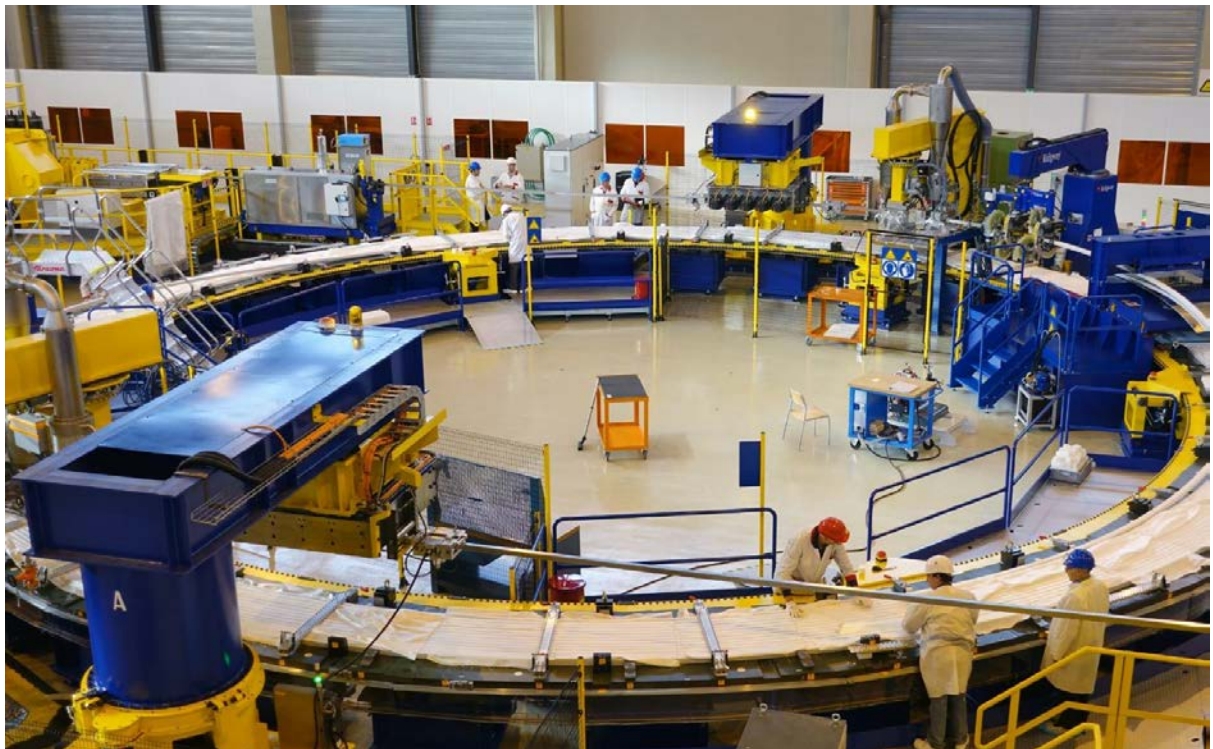
Figure 3: Preparations to wind the largest superconducting Poloidal Field coils underway on part of the production line at the ITER site
