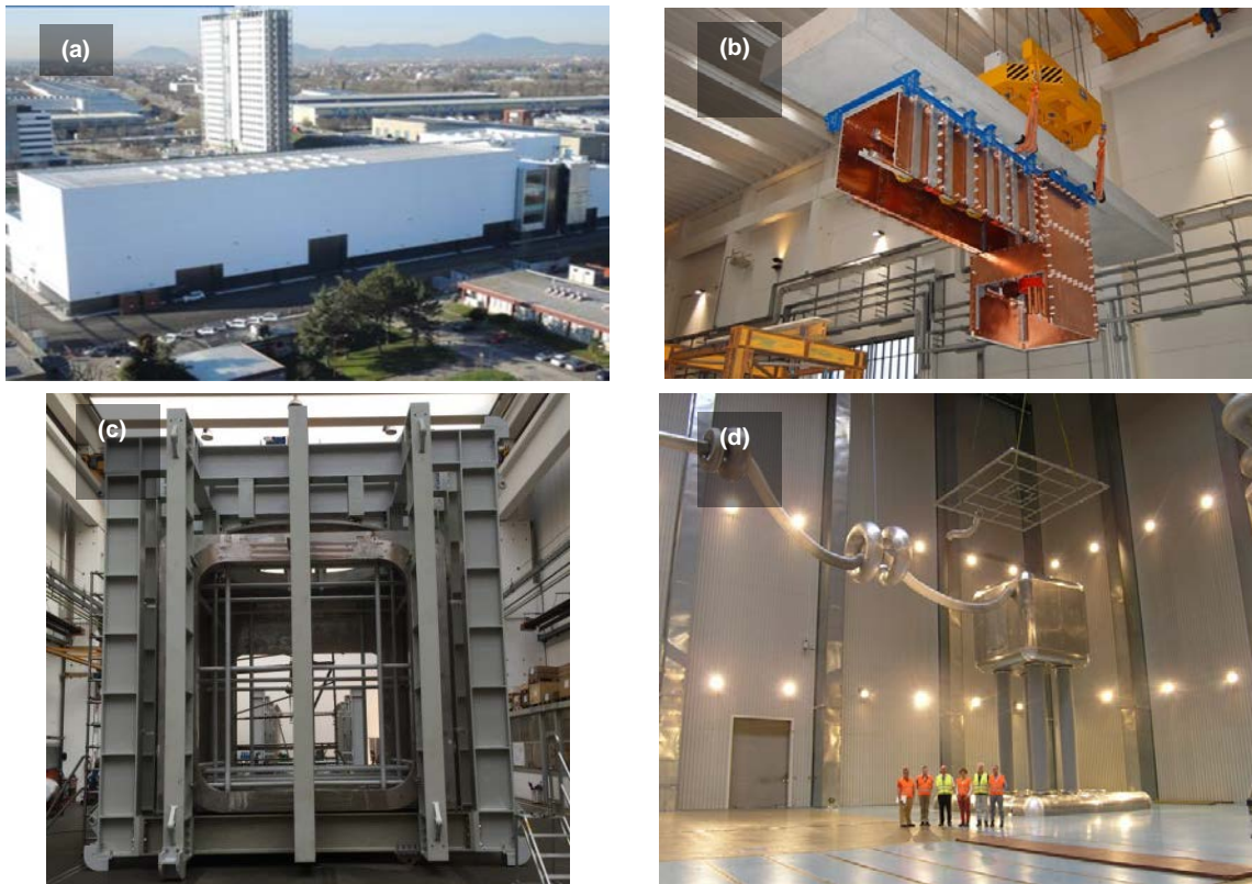
Figure 5: a) Neutral Beam Test Facility in Padua, Italy, (b) the Transmission Lines for SPIDER, (c) the MITICA Vacuum Vessel and (d) high-voltage testing of MITICA's Deck at Siemens
