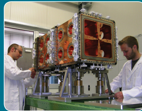
Assembly of modules for the high power testing of RF quadrupole elements at INFN
