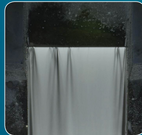
Flowing lithium in the ELTL facility (Oarai)
