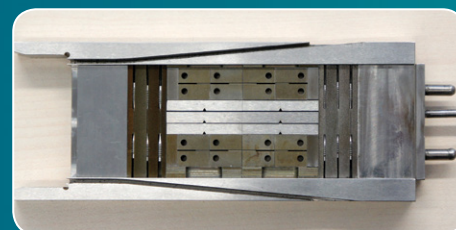
Small specimen tray (4 x 8 cm) for test irradiation (KIT, SCK-CEN)
