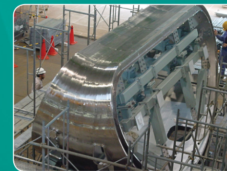
40° sector of vacuum vessel, in the Vacuum Vessel Assembly Building at the Naka Fusion Institute
