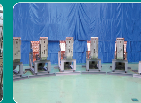
Divertor cassette bodies before mounting with plasma-facing components
