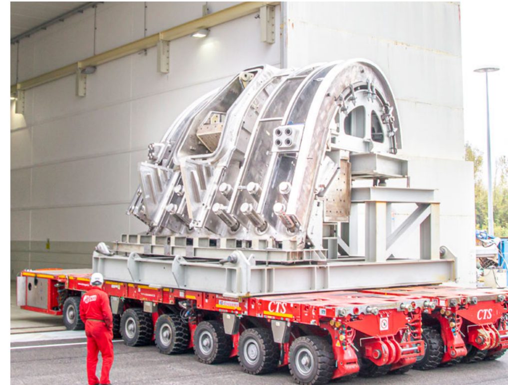
Lower segment of sector 5 of the ITER Vacuum Vessel loaded on a trailer to go through radiographic tests. Works performed in Mangiarotti, located in Monfalcone, Italy.
