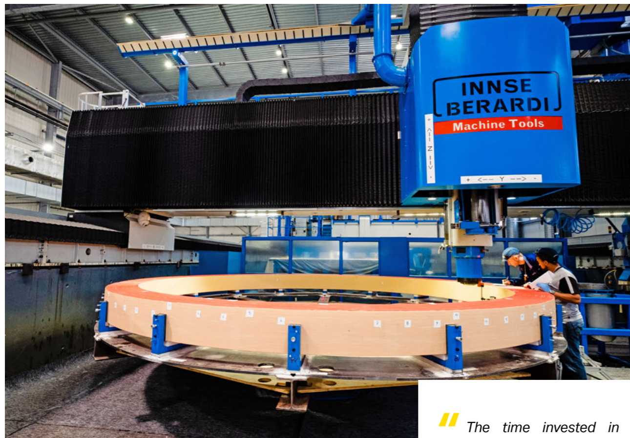
Technicians carrying out checks on the first ITER Pre-Compression Rings undergoing production. F4E is collaborating with CNIM for the manufacturing of the nine rings which will absorb the fatigue and deformation felt by the ITER Toroidal Field (TF) coils.
