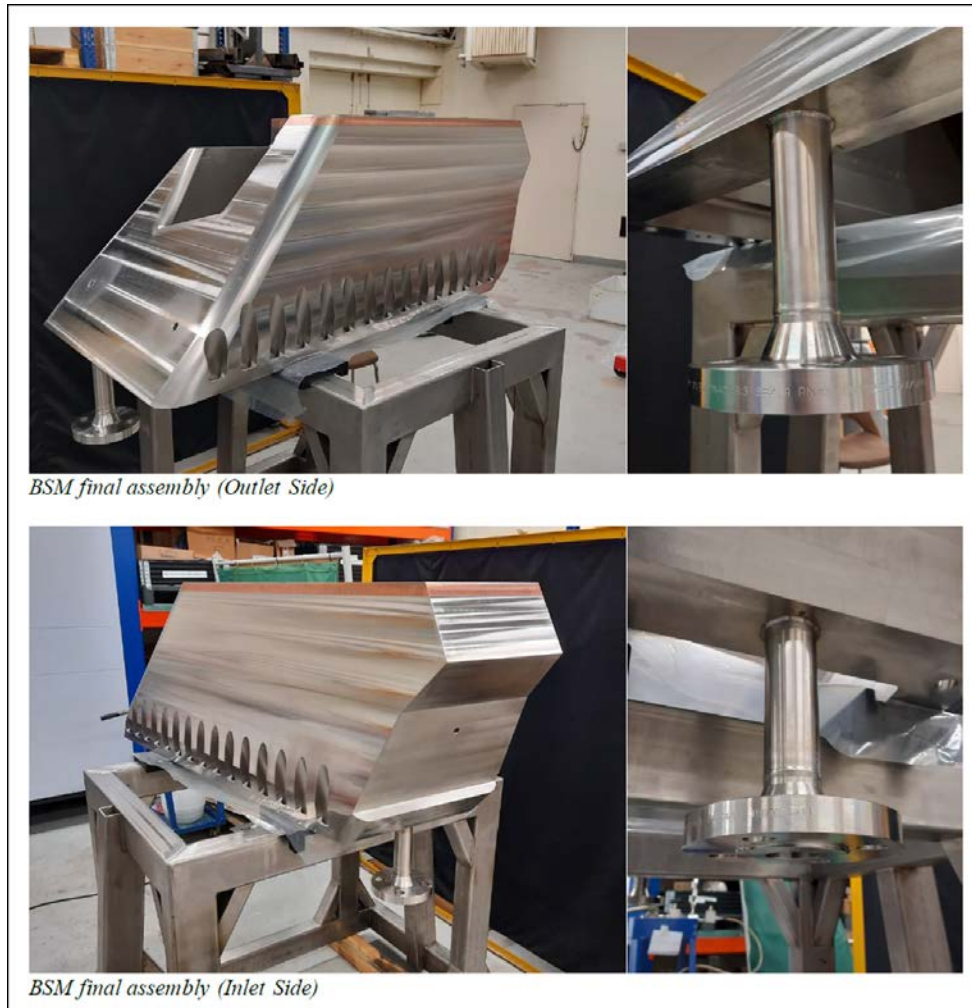
Figure 49: Further validation of the diffusion bonding process for plasma-facing blanket shield module
