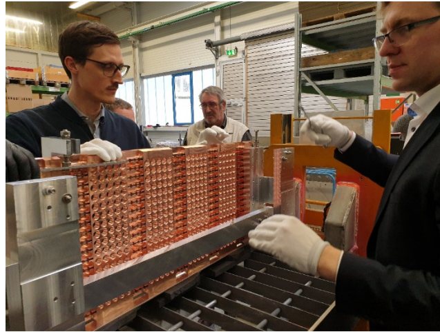
Figure 40: MITICA BS: accelerator grid segment prototype after final leak test in vacuum
