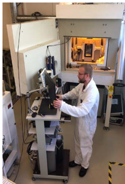
Figure 62: Testing performed after neutron irradiation up to 3 dpa at 500°C of Eurofer97 for the F4E TBM team at facilities at Studsvik AB (F4E-OFC-413-Lot3).
