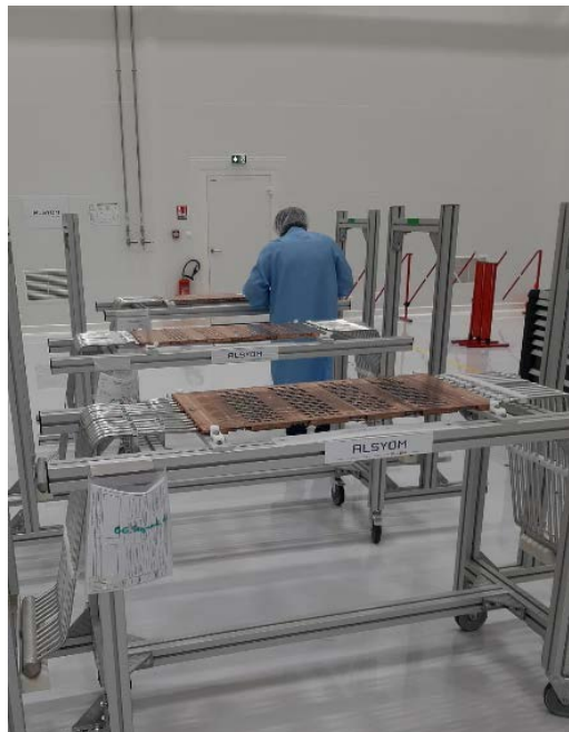
Figure 39: MITICA BS: Grids assembly
