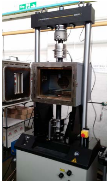
Figure 61: Customized tensile test machine with heating furnace that was later assembled in a Hot Cell
