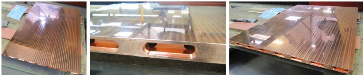
Figure 41: BLCs prototyping: deep drilling (Neutralizer panels made of Cu OF)
