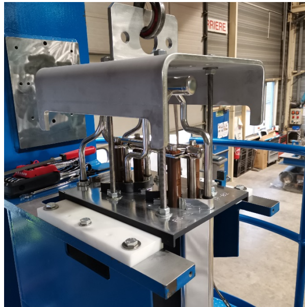
Figure 23: Leak test of a MITICA cryopump pumping section
