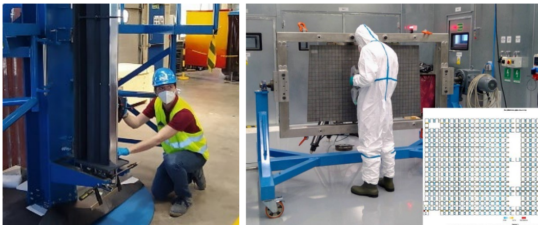
Figure 35: Dimensional Inspection Survey for the MITICA Pumping Section Qualification (left) and In-Vessel FWs full scale prototypes (right)
