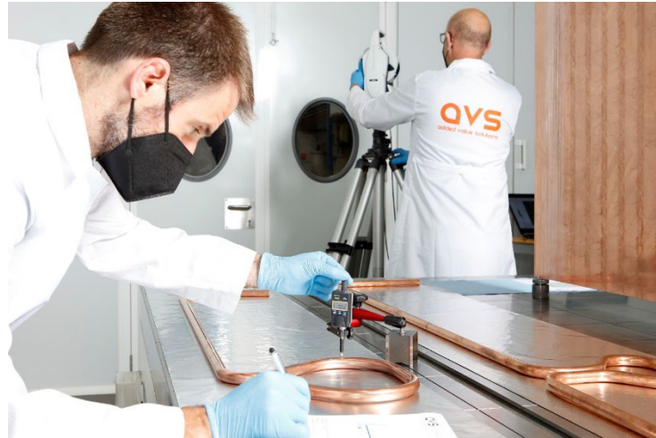
Figure 21: A swirl tube elements of the Calorimeter during the dimensional control
