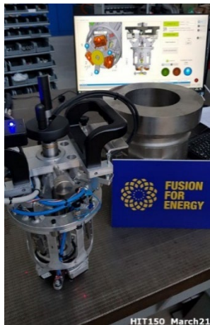
Figure 37: Ad-hoc measurement tool for VV datum reconstruction
