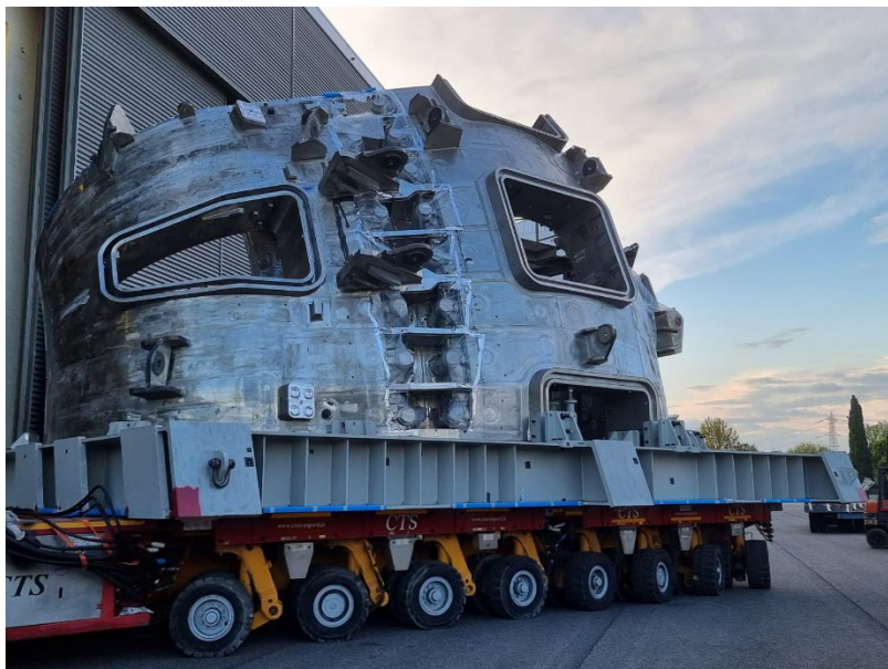
Figure 5: Sector 5 being transported to the Radiographic Test facility after completion of inner the shell welding
