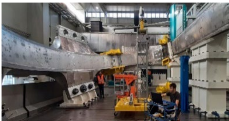
Figure 38: Dimensional Inspection Survey for the TFC FAT
