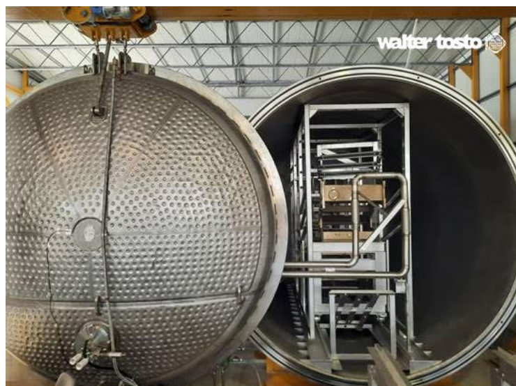
Figure 11: Hot Helium Leak Test facility at Walter Tosto premises
