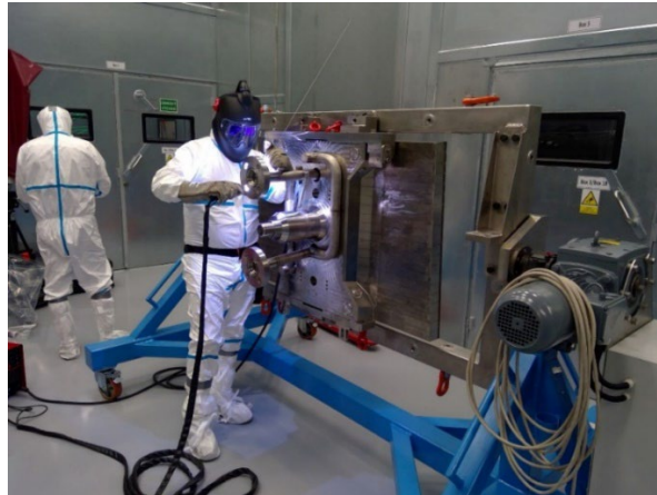
Figure 8: Successful high heat flux testing of First Wall panel Full Scale Prototypes in the CV Řez test facility at Plsen
