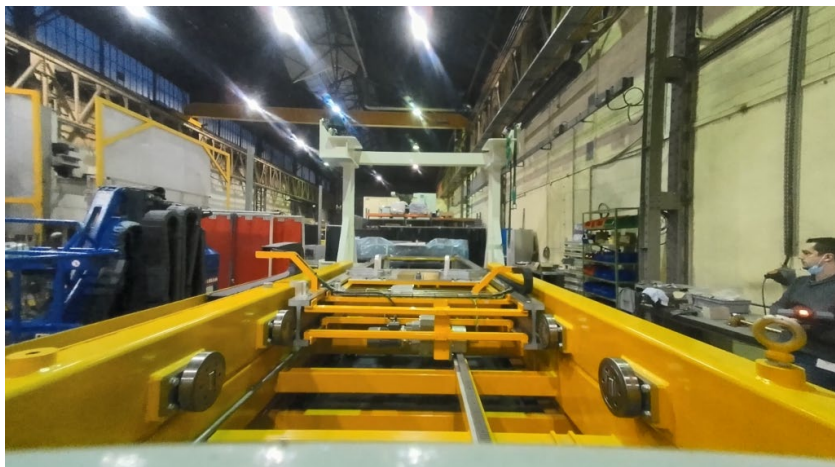
Figure 19: The Beam Source Handling Tool (BSHT) during the test on the Mock-up simulating the installation of the BS into the vacuum vessel
