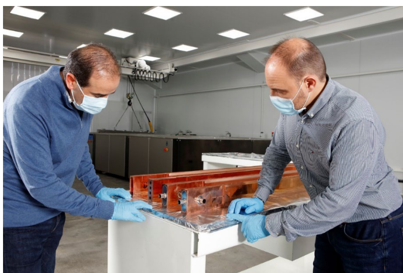
Figure 20: Four beam stopping elements for the residual ion dump at different stages of the manufacturing cycles
