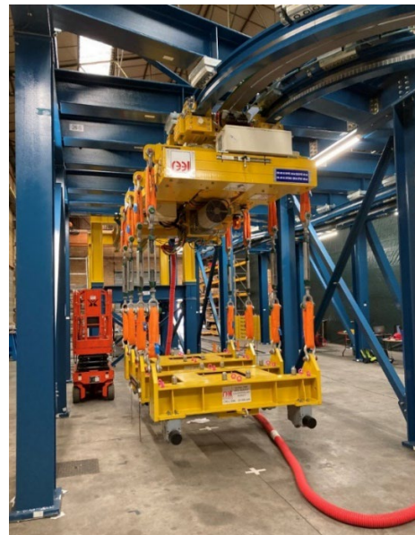
Figure 14: IVVS optical probe prototype (left) under assembly in the laboratory. NBRHS crane prototype (right) under test
