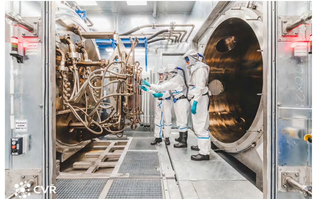
Positioning shielding frames on test sample, HELCZA Facility. © CVŘ
