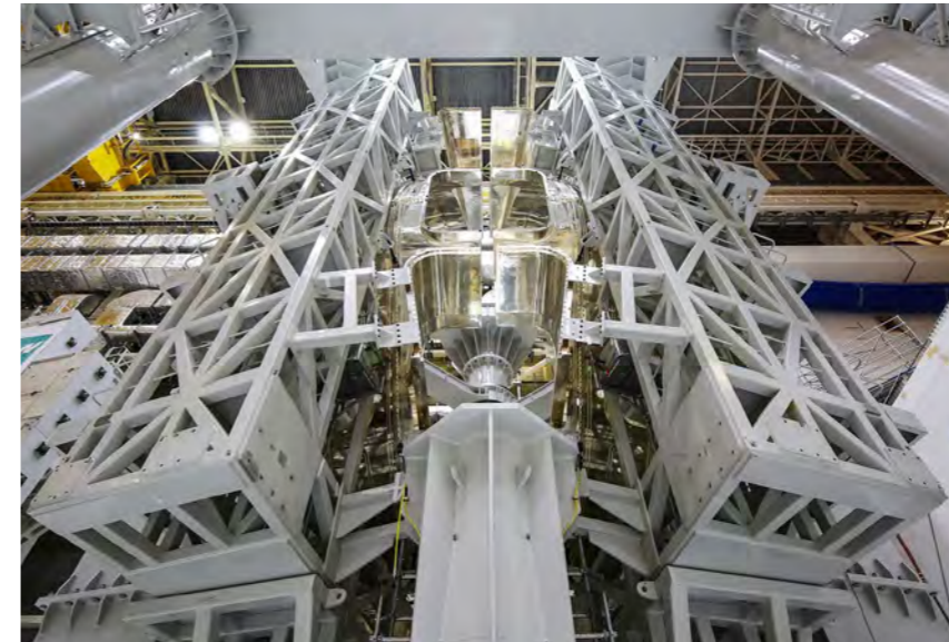
Thermal shield fitting tests carried out on sector sub-assembly tool 2, February 2021 © ITER Organization
