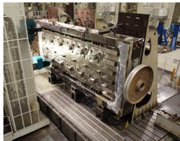
First segment of sector 5 of the ITER Vacuum Vessel, manufactured in Europe, placed on the jig in the factory of Mangiarotti, Italy, June 2021. Poloidal segment 1 manufactured by Mangiarotti © F4E
