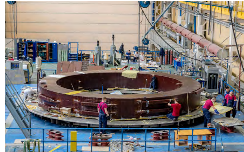
Impregnation completed for ITER Poloidal Field coil 1, Sredne-Nevisky Shipyard in St. Petersburg, Russia. 2021 © Rosatom
