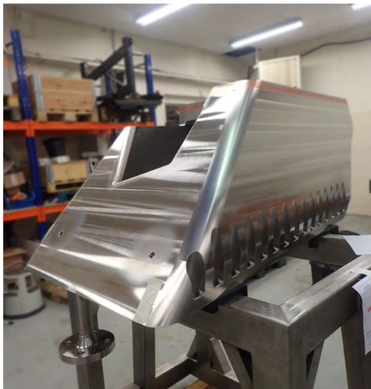
First prototype of ITER Blanket Shield Module (BSM) successfully fabricated by ATMOSTAT. © ATMOSTAT
