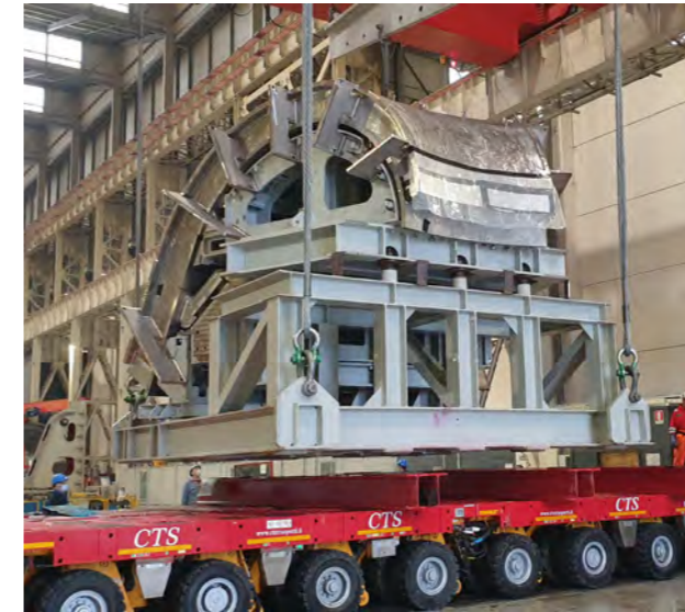
Another segment of sector 5 of the ITER Vacuum Vessel, poloidal segment 4, manufactured in Europe, lifted to be moved to the jig in the factory of Mangiarotti, Italy, June 2021. © F4E
