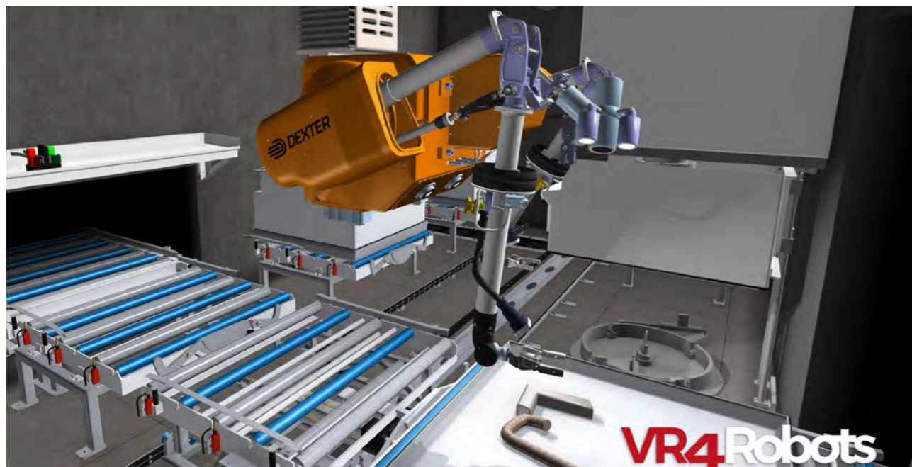
Retina remote handling simulator; a VR4Robots physics-based digital twin of Veolia Nuclear Solutions' Dexter Remote Manipulator System. © Veolia Nuclear Solutions (UK) & Tree C Technology
