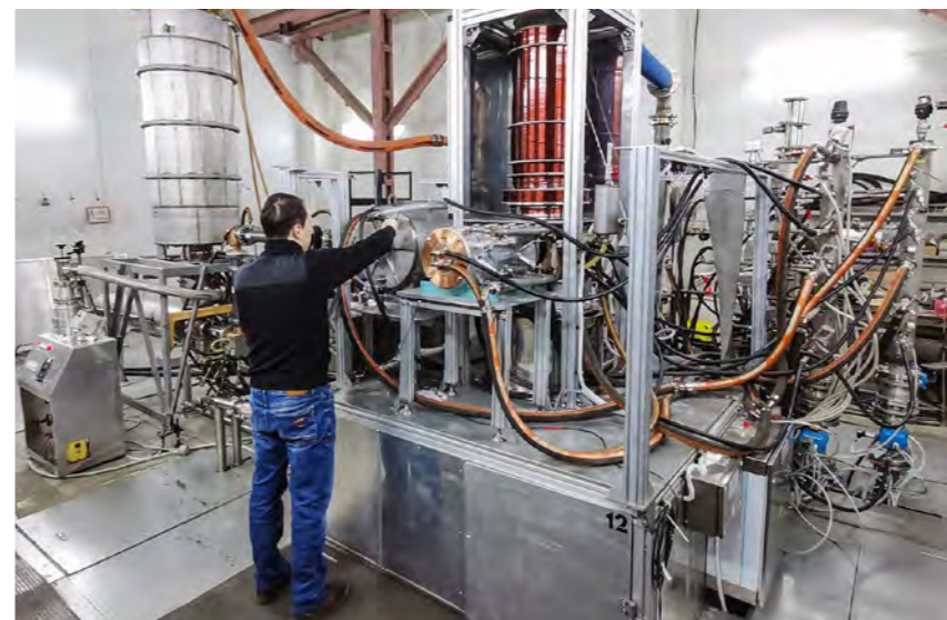
Auxiliary systems for gyrotrons sent from Nizhny Novgorod, Russia, to ITER site, Cadarache, France. December 2021 © Rosatom
