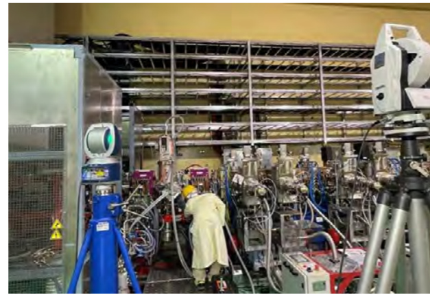
Realignment of a magnet in the Low Energy Beam Transport (LEBT) line. Japan, March 2021. © IFMIF/EVEDA
