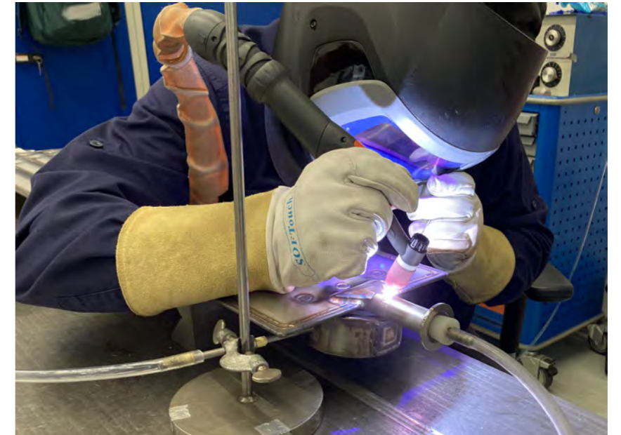
Welding the cryopanel at Research Instruments (RI), Germany, August 2021. These rectangular-shaped components measuring 1 m long and 0.2 m wide will perform the pumping by trapping the gas particles in their supercold surface. © RI
