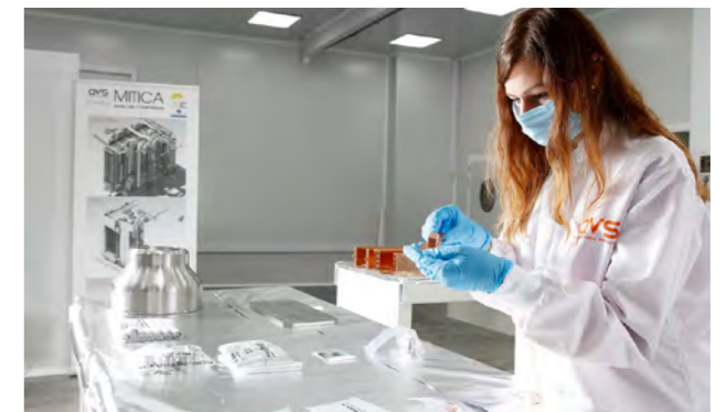
Inspection of the support pieces used for the beam stop elements, AVS, Spain, November 2021. © F4E
