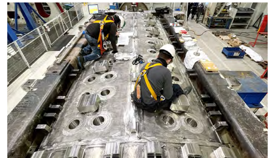
Inspector checking vacuum vessel sector 3, poloidal segment 2 at Walter Tosto, Italy, April 2021 © F4E
