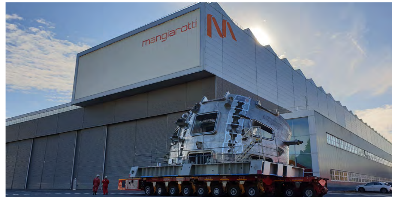
Europe's vacuum vessel sector 5 leaving the radiographic bunker of Mangiarotti to go through final tests, Mangiarotti, Italy, November 2021. © Mangiarotti
