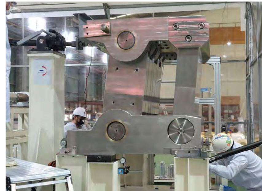
Contractors completed factory testing on the first of the nine vacuum vessel gravity supports, Korea, December 2021 © ITER Korea
