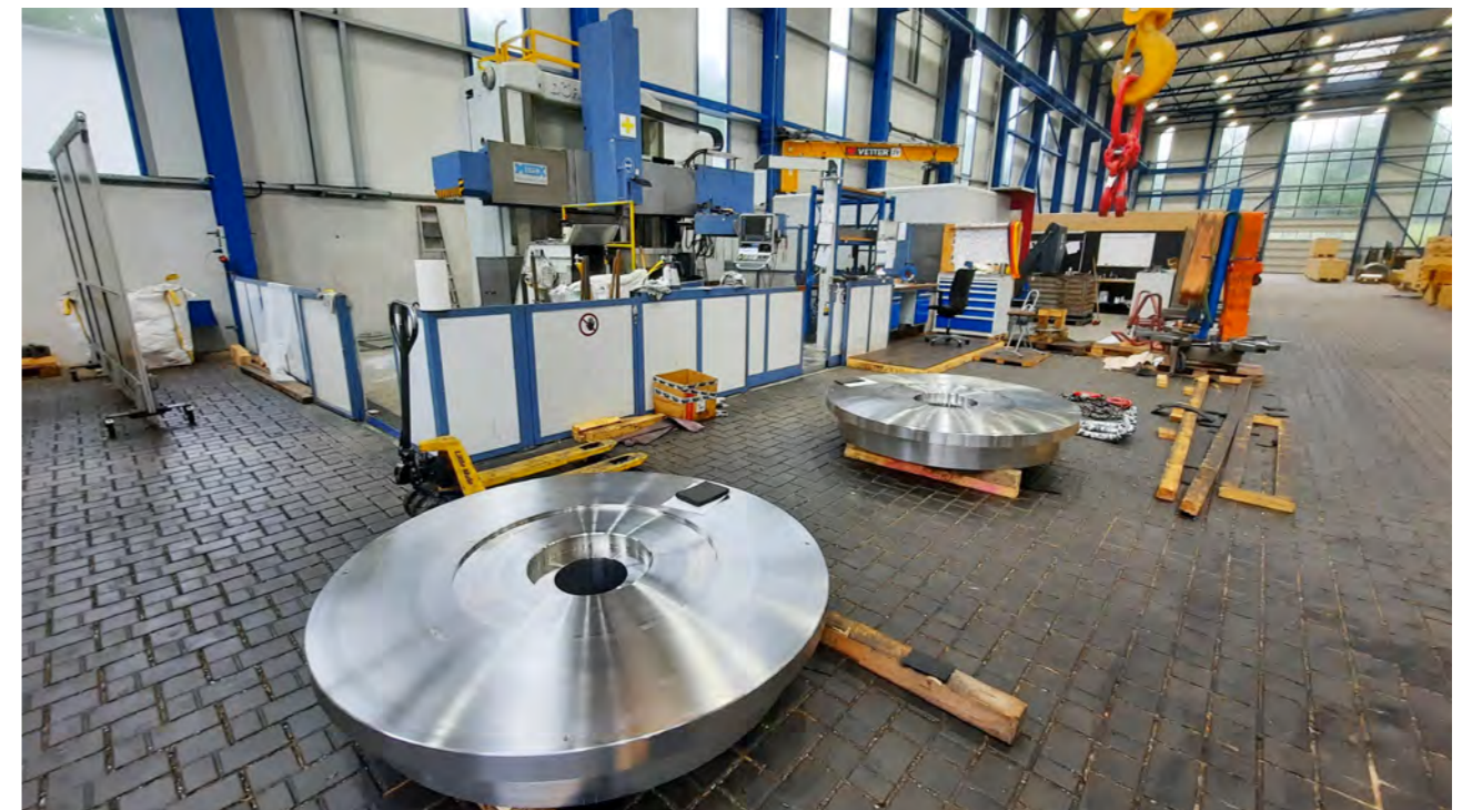
Two pump plugs in the workshop, not yet fully machined. These are the biggest components of the cryopumps. France, July 2021. © ALSYOM
