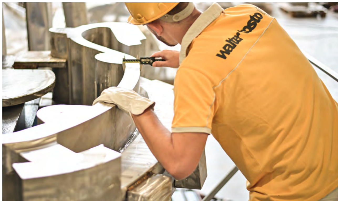
Metrology preliminary check performed on parts of ITER Divertor Cassettes bodies, Walter Tosto, Italy, September 2021. F4E has signed two contracts with Walter Tosto for the delivery of cassette bodies. © Walter Tosto
