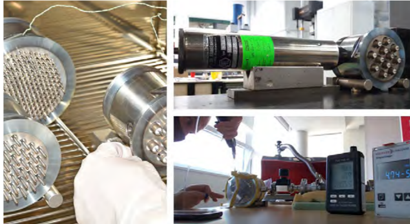
Electrical feedthrough bulkheads going through different tests. Left: thermal cycling tests; top right: impact test; bottom right: helium leak test. © Tecnia
