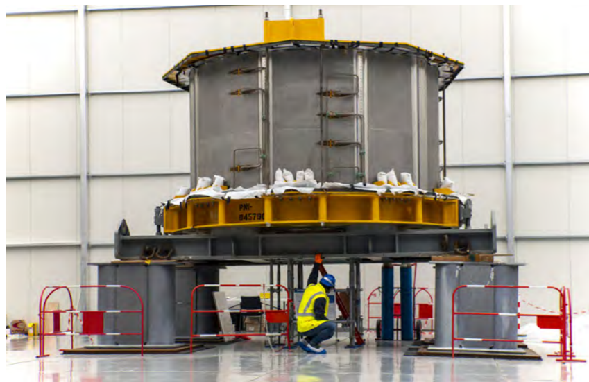
First module of central solenoid undergoing tests and verifications—metrology, sensors, electrical insulation inspection. October 2021 © ITER Organization
