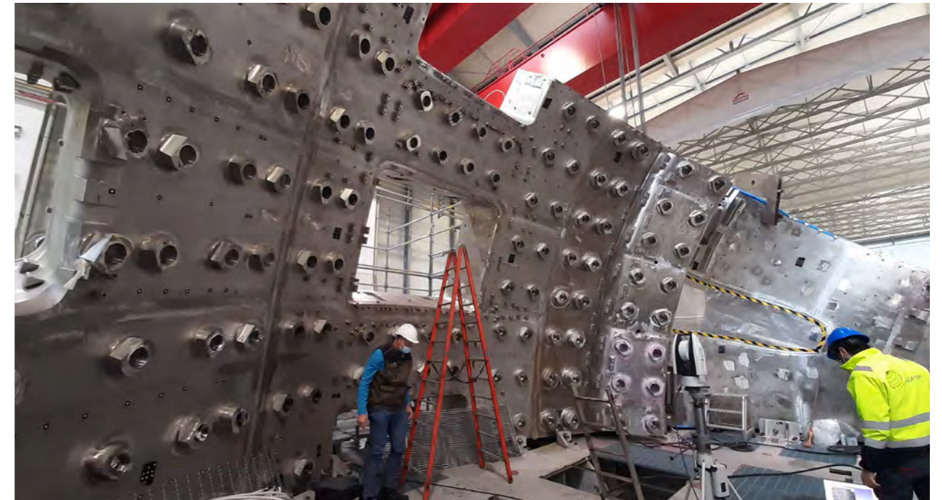
A part of ITER Vacuum Vessel sector 5, holed like a Gruyère cheese, with dozens of housings. Mangiarotti, Italy, November 2021. © F4E
