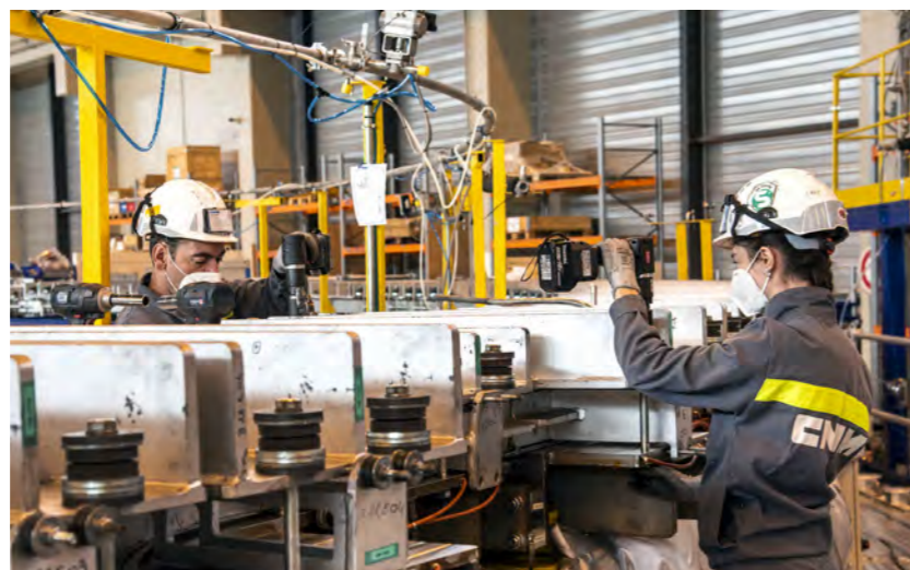
Technicians from CNIM working on the first Double Pancake of ITER Poloidal Field coil 3. Manufacturing performed in PF coils factory, Cadarache, France. © F4E
