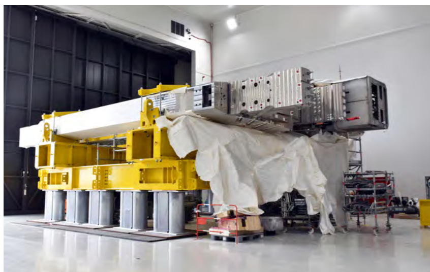
ITER Toroidal Field coil, manufactured in Japan, unwrapped in the Cleaning Facility. May 2021 © ITER Organization
