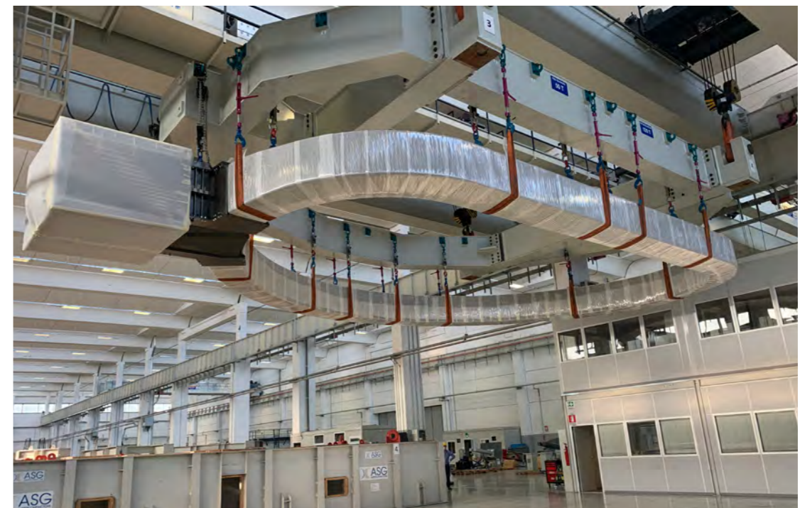
Winding packs are the inner core of the Toroidal Field coils. Pictured the last one departing from ASG Superconductors to travel by sea to SIMIC, where it will undergo final manufacturing. ASG Superconductors, La Spezia, November 2021. © F4E
