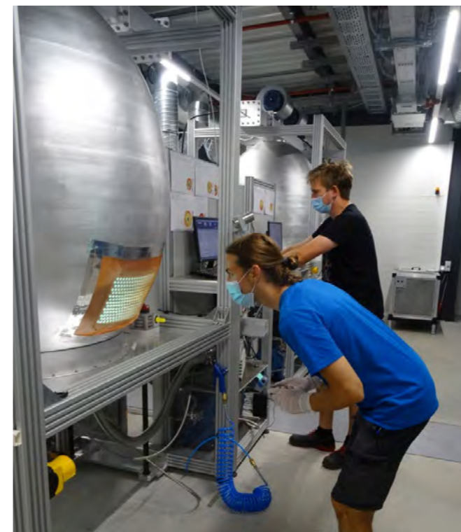
Technician in the back editing the macro that runs the machine, technician in the front inspecting the initial growth phase of diamond discs. © Diamond Materials
