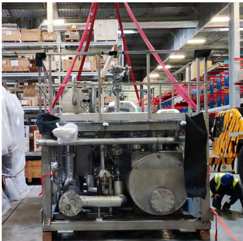
Operators unloading the warm regeneration box in the ITER premises, France, December 2021. © F4E
