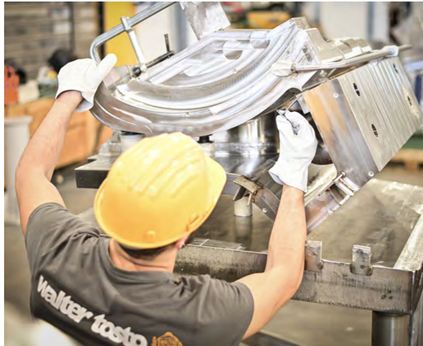
Metrology preliminary check performed on parts of ITER Divertor Cassettes bodies, Walter Tosto, Italy, September 2021. F4E has signed two contracts with Walter Tosto for the delivery of cassette bodies. © Walter Tosto
