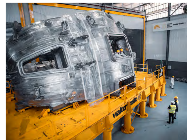
Final assembly of Europe's sector 4 of the ITER Vacuum Vessel, Walter Tosto, Italy, May 2022. ©F4E
