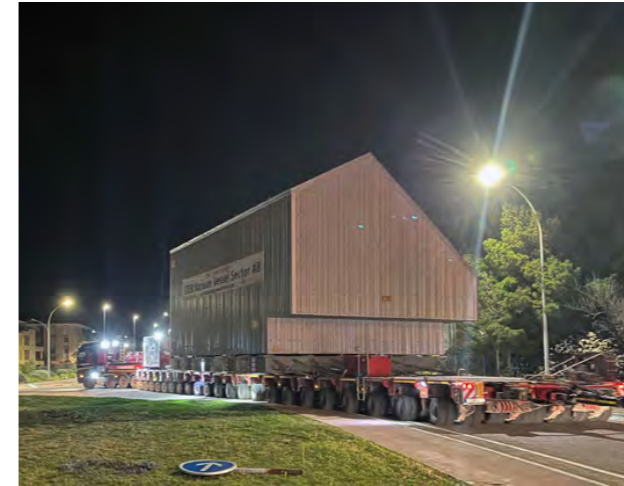
Vacuum vessel sector #8, from Korea, travelling at night along the ITER Itinerary. March 2022 ©ITER Organization
