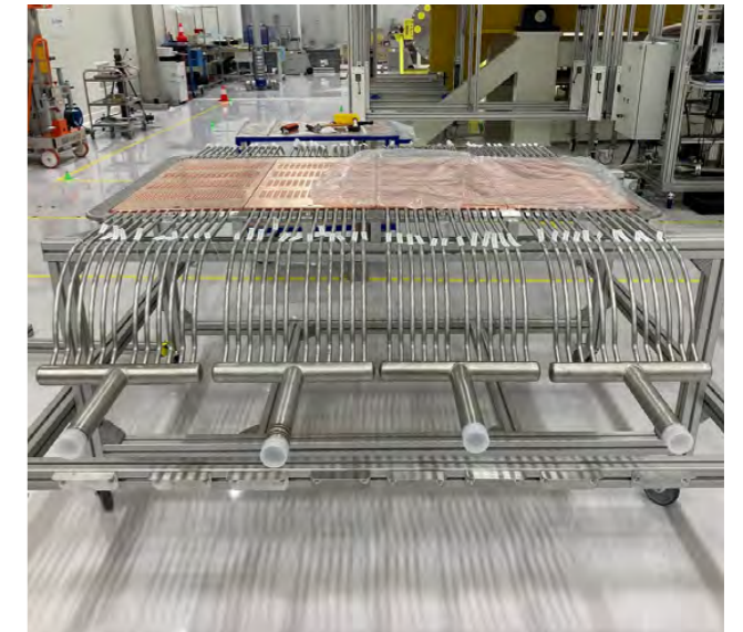
Segments of the MITICA beam source accelerator components prior to being assembled, Alsymex, Tarbes, France, May 2022. ©Alsymex
