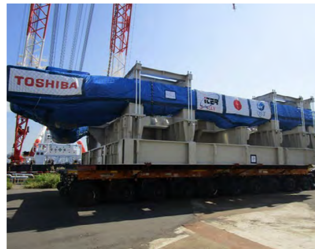
Japan's Toroidal Field coil #15, manufactured by Toshiba Energy Systems & Solutions, loaded on a barge to reach the ITER site. September 2022 ©ITER Organization
