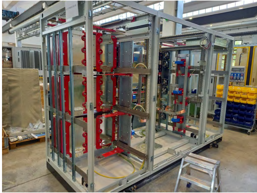
Figure 31: Manufacturing of the inverters for the Conversion System of the Acceleration Grid Power Supply of ITER
