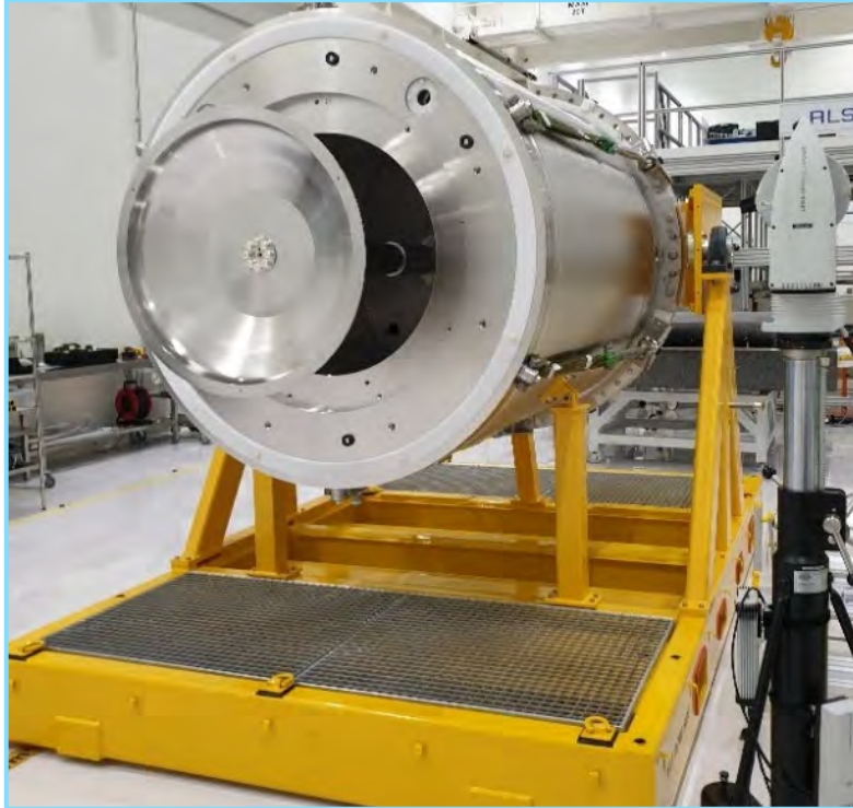
Figure 22: Torus and Cryostat cryopump – Casing and valve assembly
