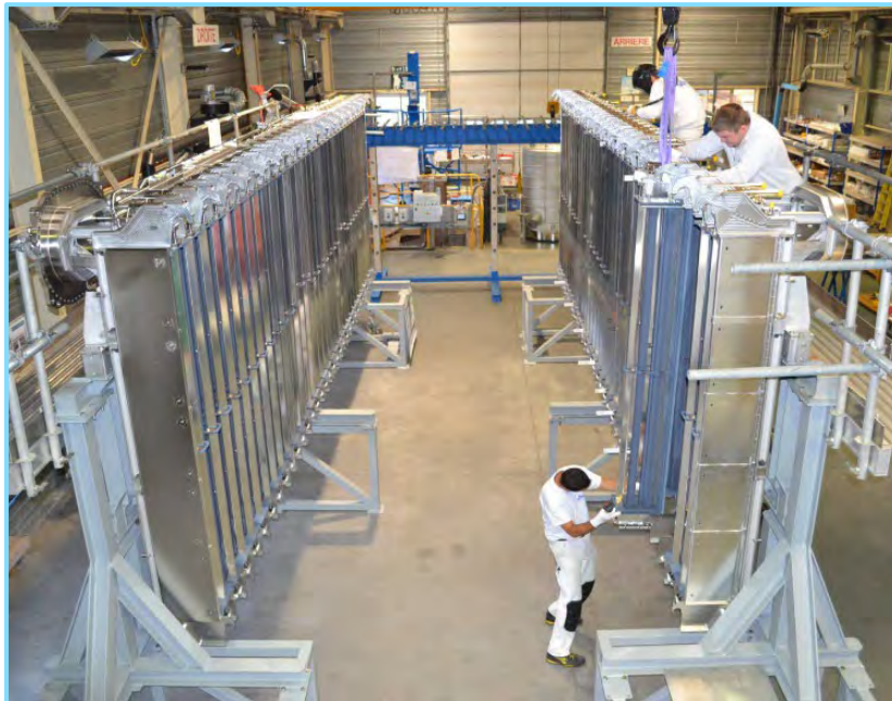
Figure 20: MITICA cryopump – final assembly stage
