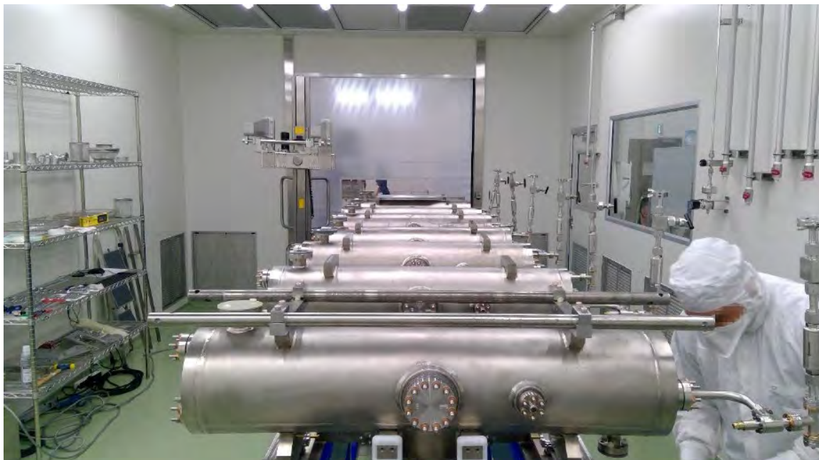
Figure 42: All 8 cavity-coupler assemblies mounted on the support frame
