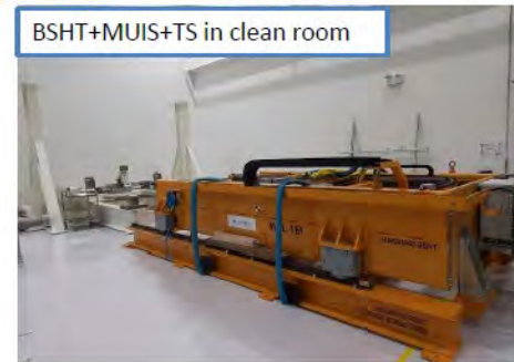
Figure 26: The main sub-assemblies of the MITICA Beam Source completed in 2022 (MUBS: Mock-Up of the Beam Source, BSHT: Beam Source Handling Tool, MUIS; Mock-Up of the Installation, TS: Tilting System, SADS: Supporting and Adjustment System)
